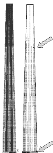
Figure 7: Longitudinal section of the reinforced chimney, and rotational symmetry angle of the reinforcement ( 45^\circ ).
