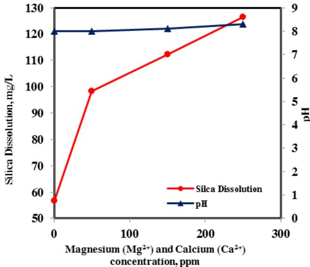
Fig. 4 The effect of Mg<sup>2+</sup> and Ca<sup>2+</sup> ions on silica dissolution using crash core samples at 80°C
