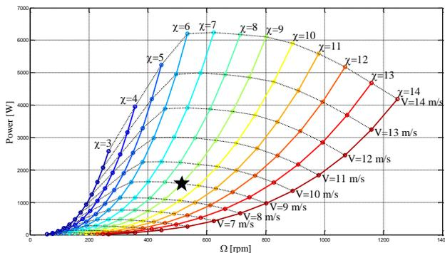
Figure 6. P- $\omega$  map with design point indication.
