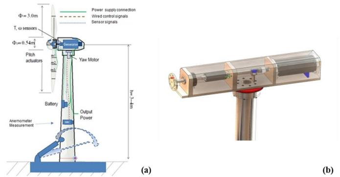
Figure 2. (a) Mini wind turbine architecture; (b) Nacelle 3D model.
