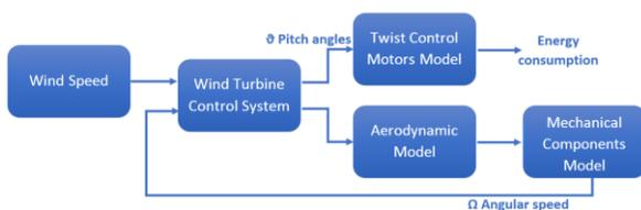
Figure 9. Wind turbine simulator scheme.
