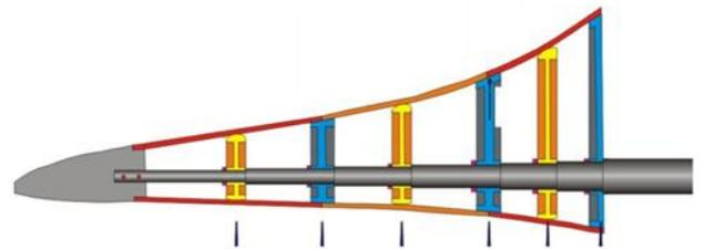
Figure 4. Blade and ribs structures with the actuation scheme (blue ribs are actuated, yellow ribs are dragged).
