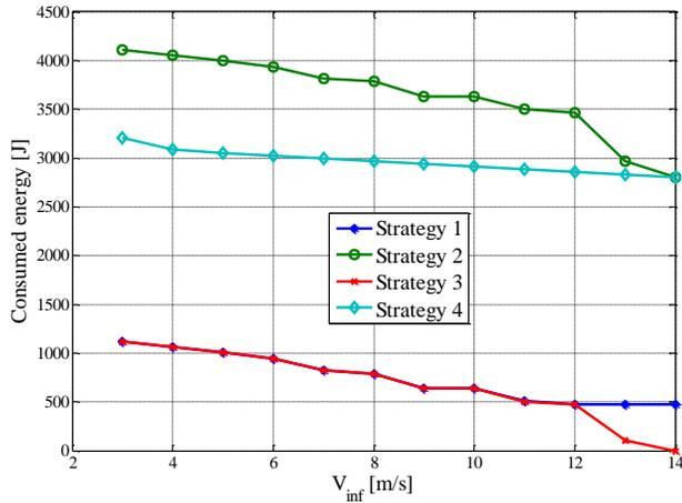
Figure 11. Test 1. Energy consumption vs. wind speed for different strategies.
