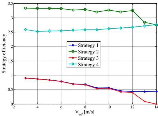
Figure 12. Test 1. Efficiency vs. wind speed for different strategies.
