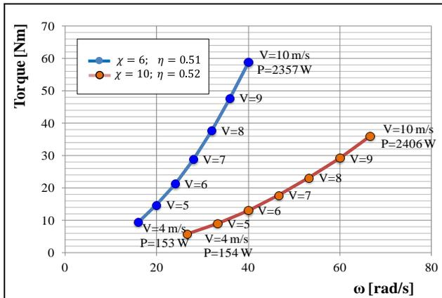
Figure 1. Aerodynamic efficiency for different values of the working ratio  $\chi=(\omega \cdot R)/V$  for different wind speed values  $V$ .
