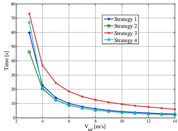
Figure 10. Test 1. Start-up time vs. wind speed for different strategies.
