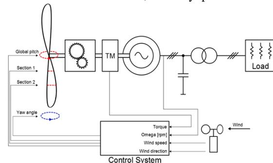
Figure 5. Block scheme of the active control loop.
