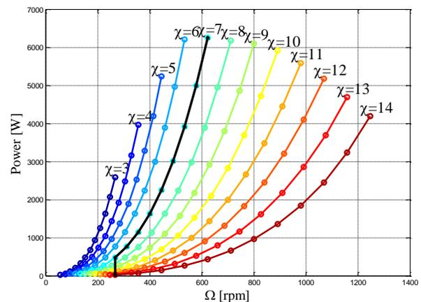
Figure 7. P- $\omega$  map with design point indication.
