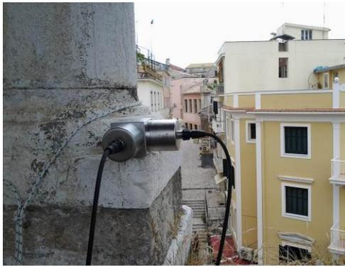
Fig.5. Two monoaxial accelerometers positioned at the base of a column of an arched-window of Annunziata bell tower.
