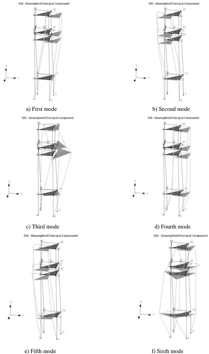
Fig.14. Mode shapes identification by using SSI method for test 2-4.
