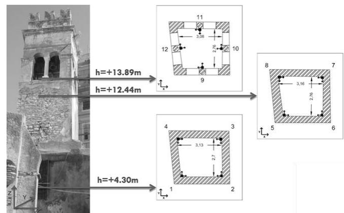
Fig. 4. Annunziata bell tower and layout of the experimental setup.
