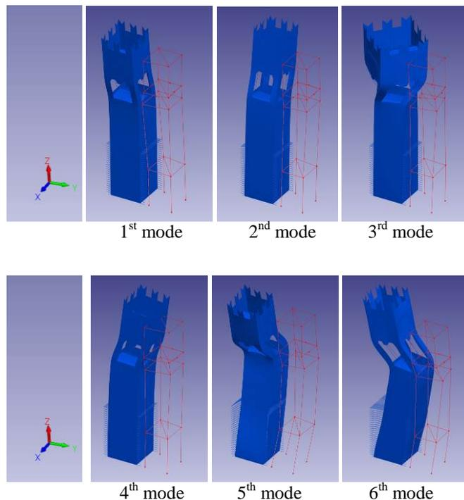
Fig. 17 Comparison between the first six theoretical (blue) and experimental (red) mode shapes.
