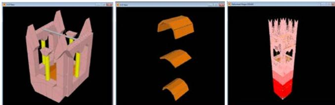
Fig.15 a) detail of the columns b) details of the vaults c) FE model.
