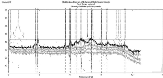
Fig.12. Identification by using SSI for test 2-4.
