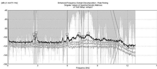
Fig.13. Identification by using EFDD for test 2-4.
