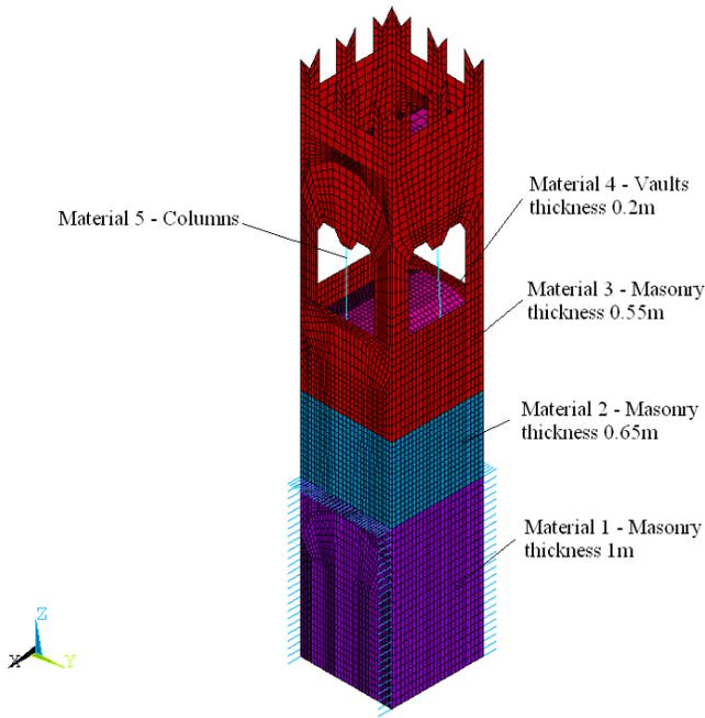
Fig.16. Numerical model used for the structural analysis: mesh and identification of material used.
