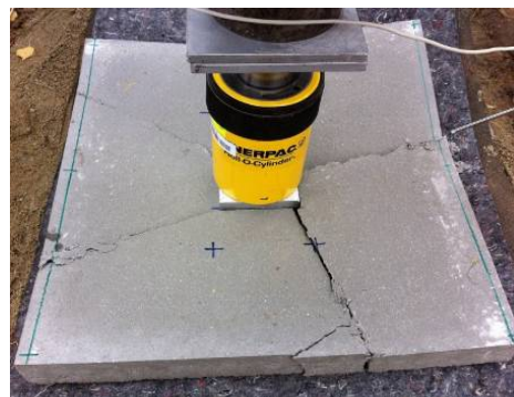
Fig. 5 Failure of the slab
