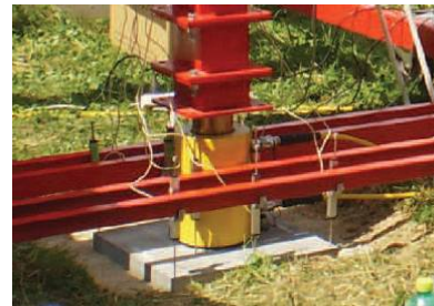
Fig. 4 Load testing of the slab
