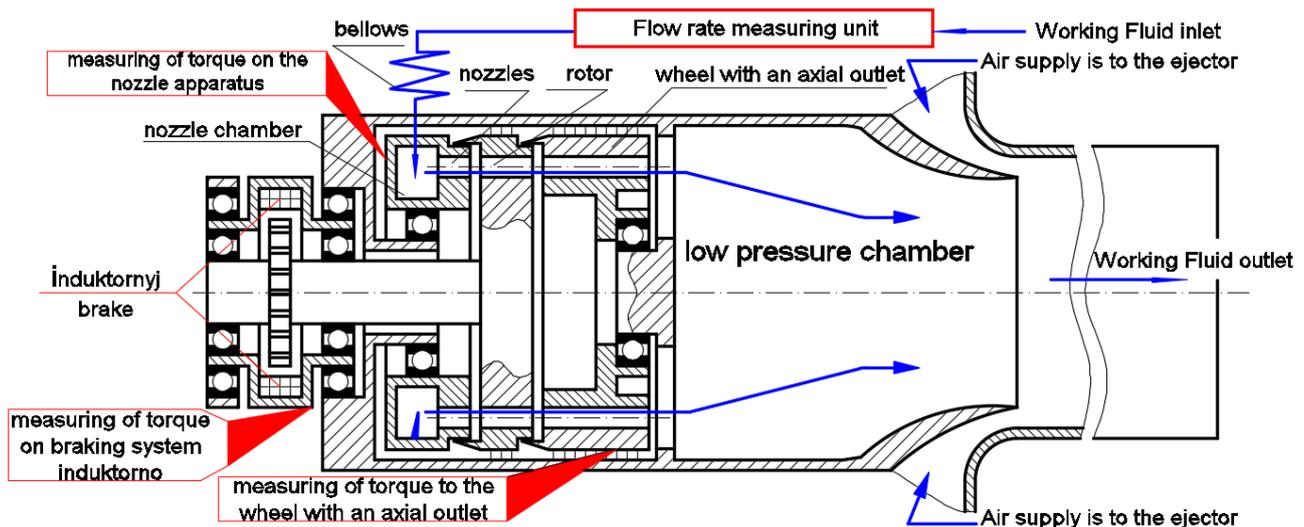
Figure 1 – Scheme of experimental stand
