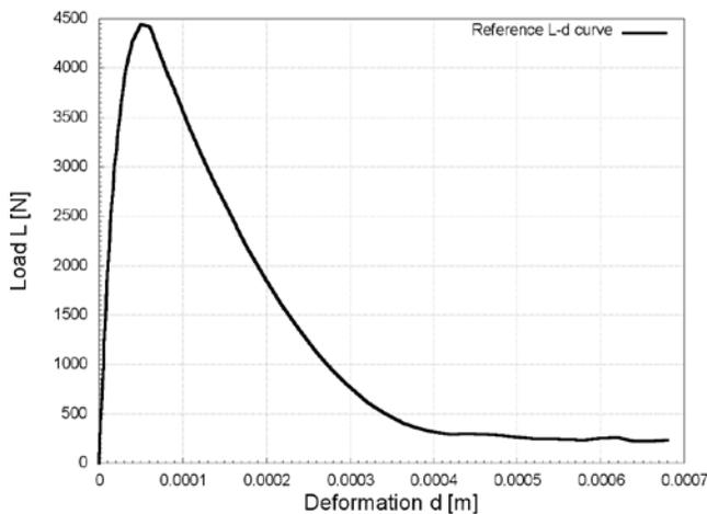
Fig. 2 Reference  $L$ - $d$  curve from a three-point bending test
