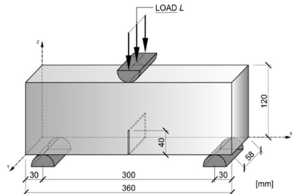
Fig. 1 Scheme of testing configuration
