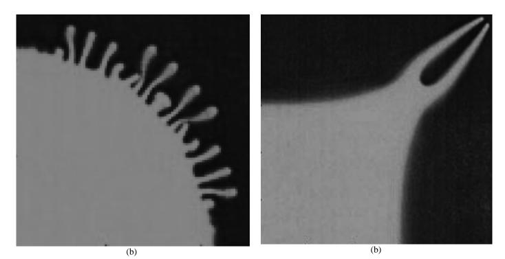
Fig. 12. Saffman-Taylor instability of the front of flooding for the five-point scheme.
