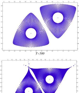
Fig. 5. The oil-water boundary for the four-spot pattern at time T=500 and T=700.
