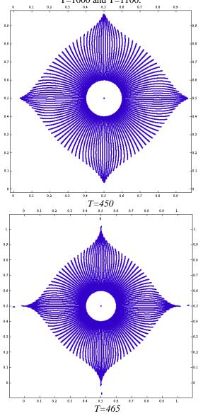
Fig. 7. The oil-water boundary for the nine-spot pattern at time T=450 and T=465.
