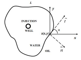
Fig. 10. Line of discontinuity L for the tangential  $V_t$  and normal  $V_n$  components of the filtration velocity.
