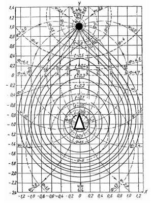
Fig. 8. The oil-water boundary as well the stream lines from injection to production well, calculated by M. Muskat [15]
