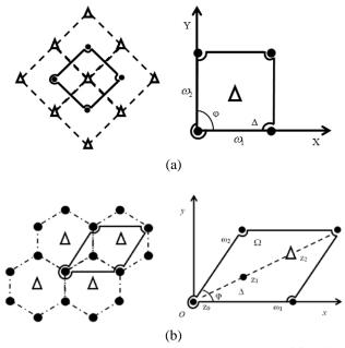
Fig. 3. Five-spot (a) and seven-spot (b) patterns of flooding (production wells are marked by black circles, injection - by white triangles) and corresponding doubly periodic lattice  $\Omega$
