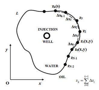
Fig. 11. Parameterization scheme of line *L* and its discretization by points  $Z_k$  ( $k = 0...N^{-1}$ ).
