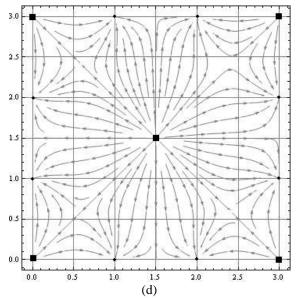
Fig. 4. The stream lines for five-spot (a), seven-spot (b), ninespot (c) and thirteen-spot (d) patterns of waterflooding [24].
