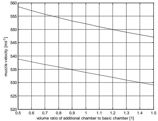
Fig. 11. Muzzle velocity vs. ratio of additional chamber volume to basic chamber volume (robust solution – solid line, simplified solution – dotted line).
