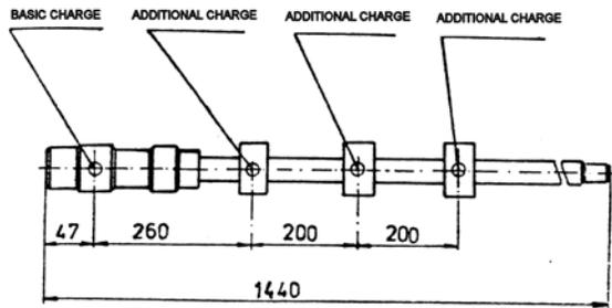
Fig. 3. Chambers placement alongside the barrel bore.
