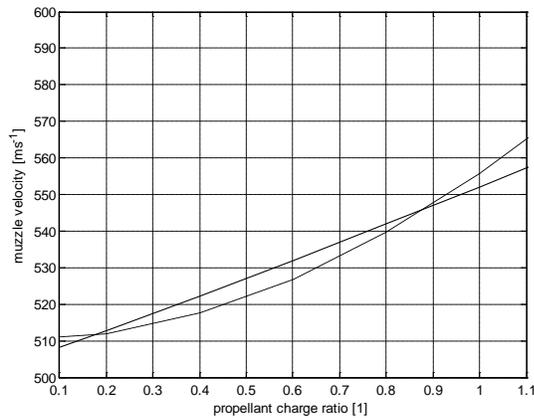
Fig. 13. Muzzle velocity vs. ratio of mass of additional propellant charge to basic charge (robust solution – solid line, simplified solution – dotted line).
