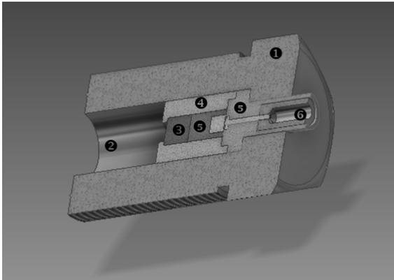
Fig. 4. The additional charge assembly (1 – body of the additional chamber screw, 2 – combustion volume, 3 – initiator F3, 4 – metal casing sleeve, 5 - resin insulator casing, 6 – firing contact pin assembly).
