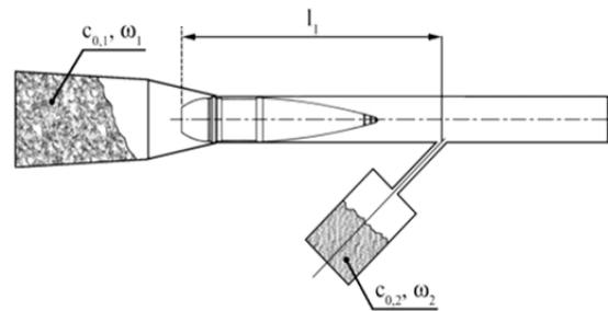
Fig. 2. Scheme of multi-chamber gun with one additional chamber.
