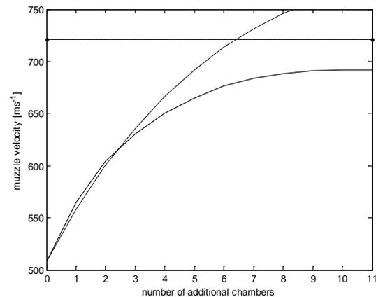
Fig. 9. Muzzle velocity vs. number of additional chambers (numerical solution – solid line, constraint value – slash-dot line, simplified formula – dotted line).
