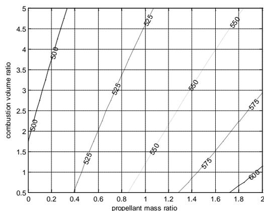
Fig. 14. Isotachs of experimental system (velocities in  $[\text{ms}^{-1}]$ ).
