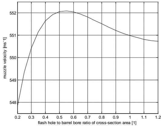
Fig. 10. Muzzle velocity vs. flash hole to barrel bore ratio of cross-section area.
