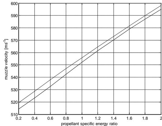
Fig. 12. Muzzle velocity vs. specific energy ratio (robust solution – solid line, simplified solution – dotted line).
