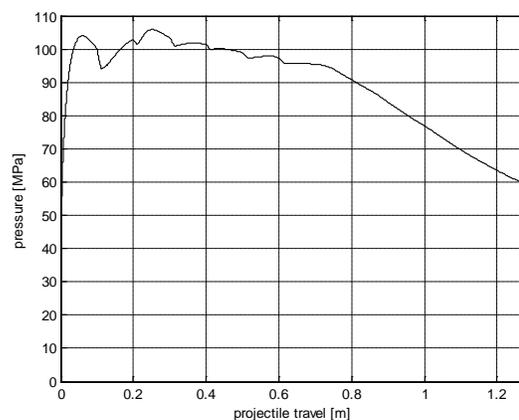
Fig. 15. Modelled pressure course of multi-chambered gun.
