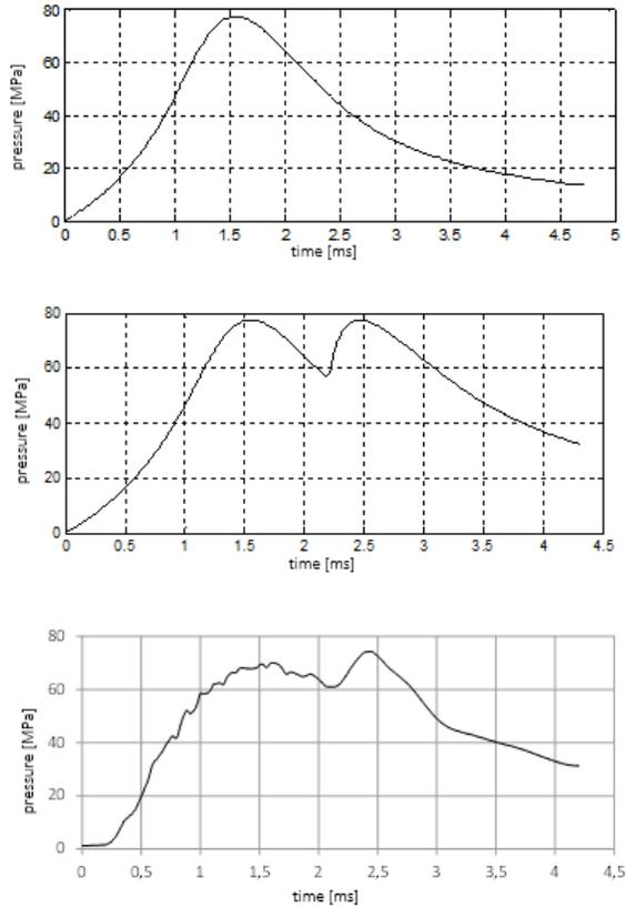
Fig. 6. Pressure courses (model of typical gun – upper, model of gun with one additional chamber – middle, measurement of gun with one additional chamber).
