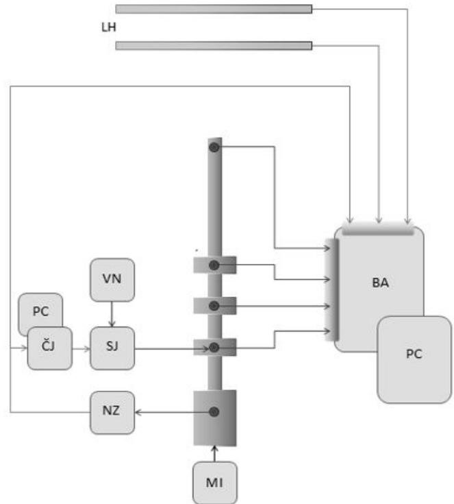
Fig. 5. The measuring chain (PC-personal computers, BA-ballistic analyzer, NZ-charge-voltage transducer, ČJ-timing unit, SJ-switch unit, VN-high voltage unit, LH-laser gates, arrows-signal lines, dots – pressure sensors).
