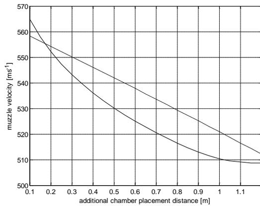
Fig. 7. Influence of additional chamber placement on muzzle velocity (numerical solution – solid line, simplified solution – dotted line).
