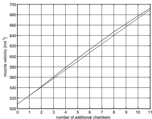
Fig. 8. Influence of evenly-spaced additional charges on muzzle velocity (robust solution – solid line, simplified solution – dotted line).
