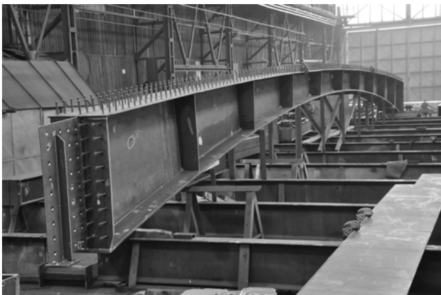
Fig. 2: Pcb girder for pedestrian bridge in Czech Republic
