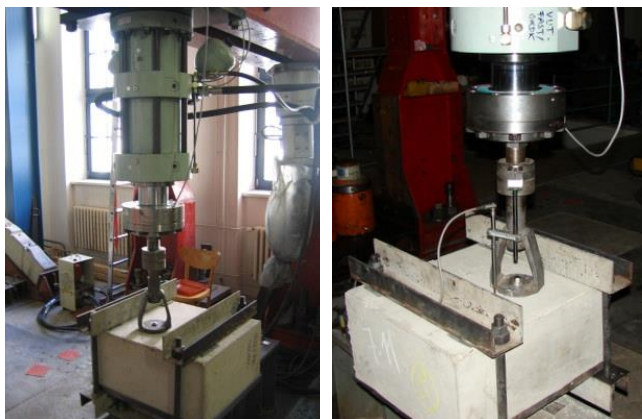
Fig. 11 illustration of the test arrangement (cylinder and loading cell)
