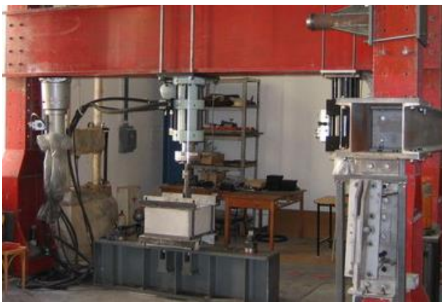
Fig. 10 illustration of the test arrangement (the steel loading frame)
