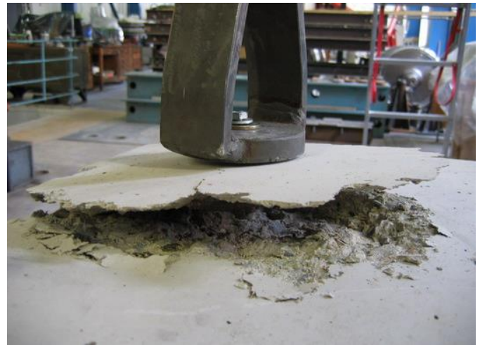
Fig. 15 failed specimen (concrete-cone failure)
