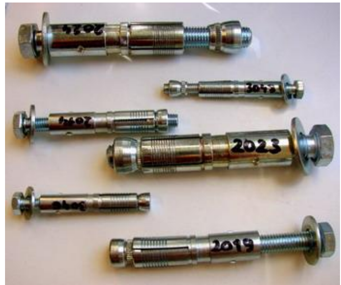
Fig. 1 type of the steel mechanical post-installed expansion anchors which have been selected for the loading tests
