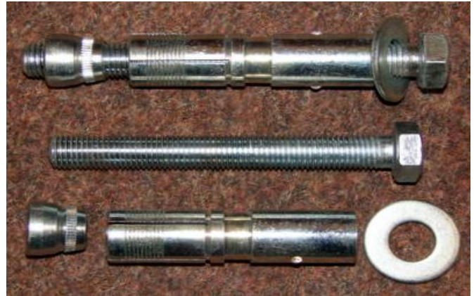
Fig. 12 steel mechanical expansion anchors used for the loading tests
