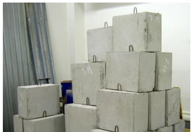
Fig. 13 concrete specimens used for the experiments
