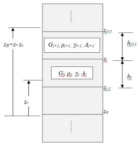
Fig. 4 A piecewise-continuous model for an *N*-layer building subjected to seismic motion below  $z_0$ .
