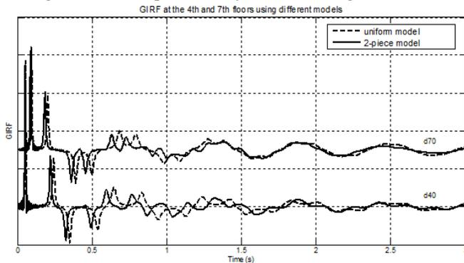
Fig. 10 Comparison of GIRFs at the 4<sup>th</sup> and 7<sup>th</sup> floor with respect to impulsive basement acceleration obtained with one- and two-layer models.
