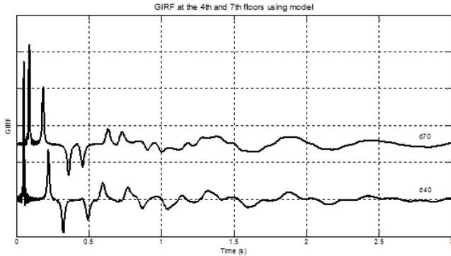
Fig 6 GIRFs at the 4<sup>th</sup> and 7<sup>th</sup> floors with respect to impulsive basement acceleration obtained based on Eqs. (10)-(12) with  $r_{11}=0.04$ ,  $v_1=345.18$  m/s,  $v_2=10.32$  m/s,  $h_1=46.98$  m,  $h_2=1.22$  m, and  $\gamma_1=\gamma_2=0.03$ .
