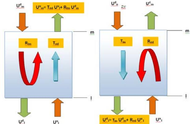
Fig 5a,b Transmission and reflection coefficients  $T_{ml}$  and  $R_{lm}$  (Fig. 5a, left) or  $T_{lm}$  and  $R_{ml}$  (Fig. 5b, right) relate the out-going wave  $U_m^u$  (left) or  $U_l^d$  (right) and input waves  $U_m^d$  and  $U_l^u$  in building segment bounded by  $(z_l, z_m)$  or  $(l,m)$
