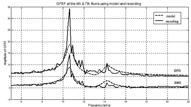
Fig. 7 Comparison of GFRF amplitudes at the 4<sup>th</sup> and 7<sup>th</sup> floors with respect to impulsive basement acceleration obtained from seismic recordings and model (Eq. (11a)).
