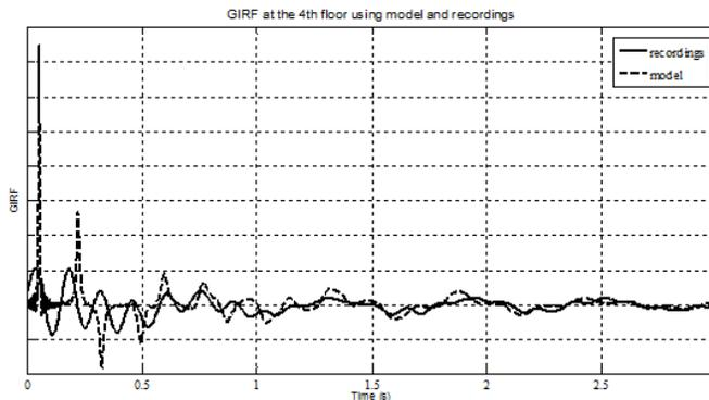
Fig. 8b Comparison of GIRF at the 4<sup>th</sup> floor with respect to basement acceleration motion obtained from seismic recordings and model (Eqs. (9b) and (11a)).
