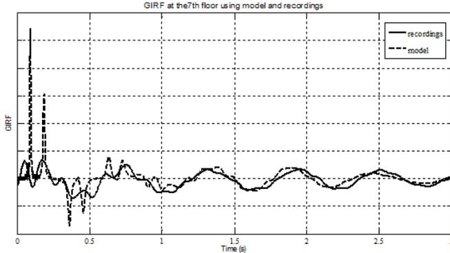
Fig 8a Comparison of GIRF at the 7<sup>th</sup> floors with respect to basement acceleration motion obtained from seismic recordings and model (Eqs. (9b) and (11a)).
