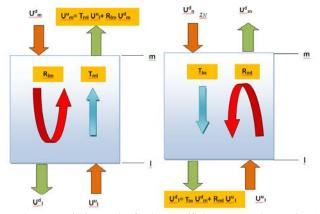
Fig 5a,b Transmission and refection coefficients  $T_{ml}$  and  $R_{lm}$  (Fig. 5a, left) or  $T_{lm}$  and  $R_{ml}$  (Fig. 5b, right) relate the out-going wave  $U_m^{u}$  (left) or  $U_l^d$  (right) and input waves  $U_m^d$  and  $U_l^u$  in building segment bounded by  $(z_l, z_m)$  or (l, m)
