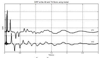
Fig 6 GIRFs at the 4<sup>th</sup> and 7<sup>th</sup> floors with respect to impulsive basement acceleration obtained based on Eqs. (10)-(12) with  $r_{II}=0.04$ ,  $v_1=345.18$  m/s,  $v_2=10.32$  m/s,  $h_1=46.98$  m,  $h_2=1.22$  m, and  $\gamma_1=\gamma_2=0.03$ .
