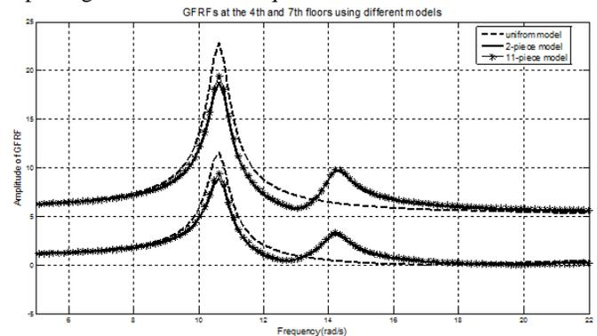
Fig. 9 Comparison of GFRF amplitudes at the 4<sup>th</sup> and 7<sup>th</sup> floors with respect to impulsive basement acceleration obtained with uniform (one-layer), two-layer and eleven-layer models from seismic recordings and models.
