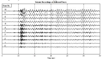
Fig. 2 Seismic acceleration recordings of Yorb Linda earthquake in the north-south direction at different floors (indicated as 0-10), where floor levels 0 and 10 correspond to B and R respectively in Fig. 1.
