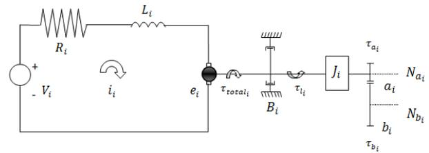
fig. 4 schematic representation of a DC motor
