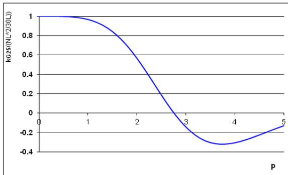
Fig. 6. The normalized consistent geometric stiffness term  $k_{G25}$ .
