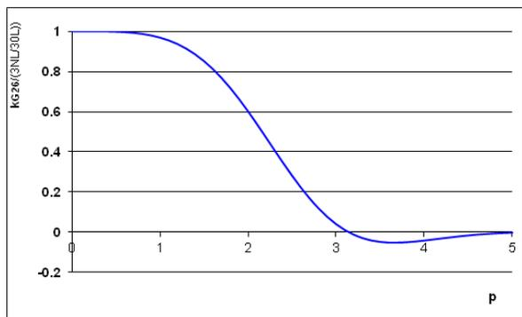
Fig. 7. The normalized consistent geometric stiffness term  $k_{G26}$
