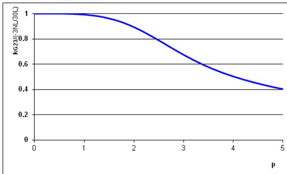
Fig. 5. The normalized consistent geometric stiffness term  $k_{G23}$
