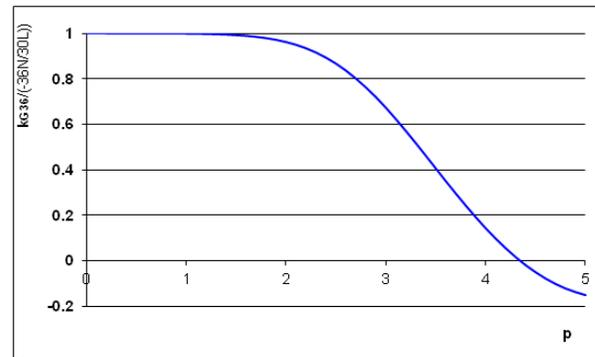
Fig. 9. The normalized consistent geometric stiffness term  $k_{G36}$
