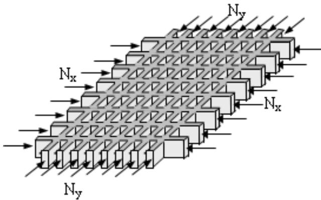
Fig. 2. The Representation of a Modal Plates by Parallel sets of one-dimensional elements replaced by the continuous surface under the action of biaxial in-plane loads.
