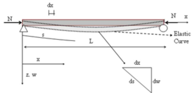
Fig. 3. The Deformed Shape of a Simply Supported Axially Loaded Beam Element.
