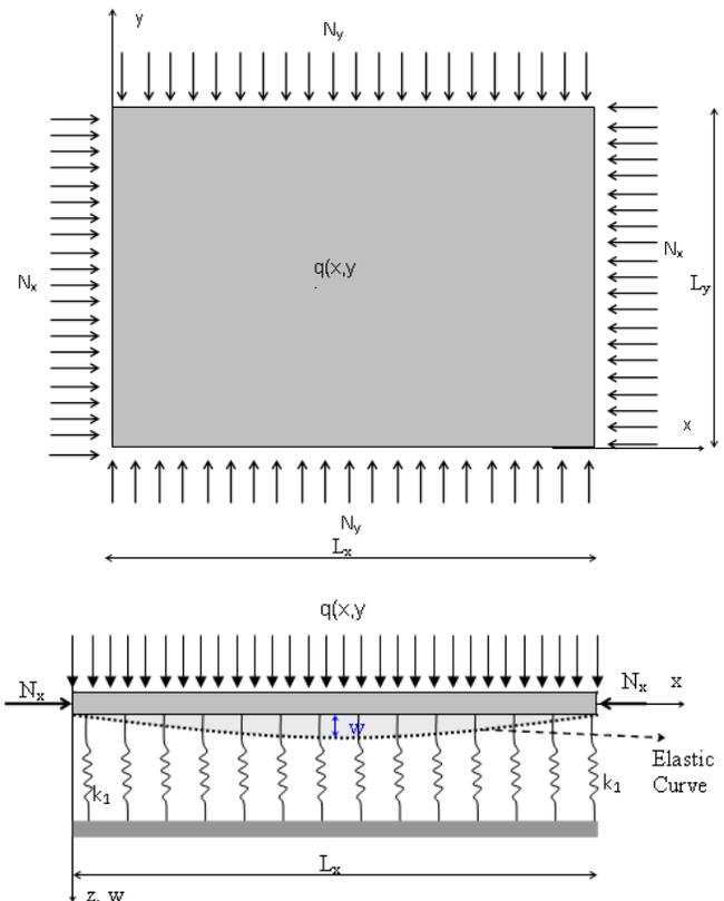
Fig. 1. The Representation of a Modal Plates Resting on Winkler Foundation Under the Combined Action of Transverse Load and Biaxial In-Plane Loads.
