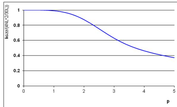
Fig. 4. The normalized consistent geometric stiffness term  $k_{G22}$
