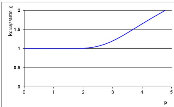
Fig. 8. The normalized consistent geometric stiffness term  $k_{G33}$
