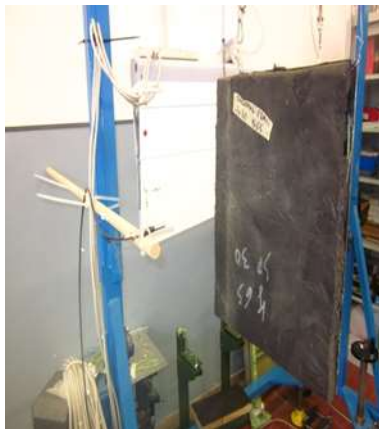
Fig. 10 Acoustic test set-up, Plate with Original Foam
