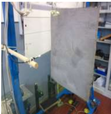
Fig. 11 Acoustic test set-up, Plate with Foam 65-30
