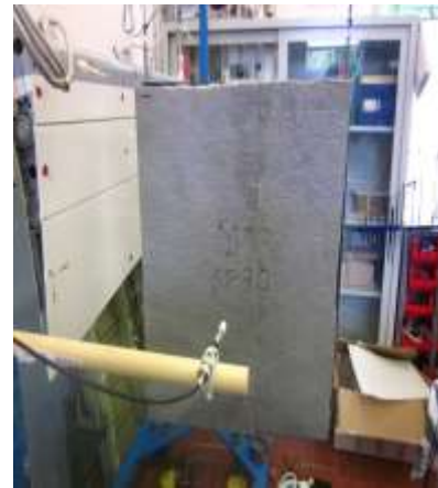
Fig. 12 Acoustic test set-up, Plate with Foam 75-30
