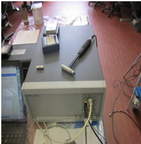
Fig. 5 Dynamic contact test instrumentation
