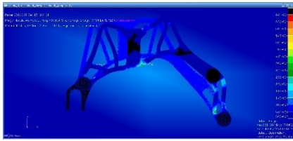
Fig. 7: Strain energy (with ROD) – mode 2
