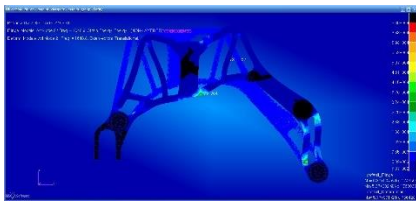
Fig. 6: Strain energy (without ROD) – mode 2
