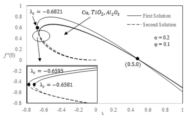
**Fig. 1.** Skin friction coefficient  $f''(0)$  as a function of  $\lambda$  for various nanoparticles.
