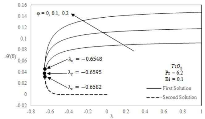
**Fig. 5.** Local Nusselt number coefficient  $-\theta'(0)$  as a function of  $\lambda$  for various values of  $\phi$ .
