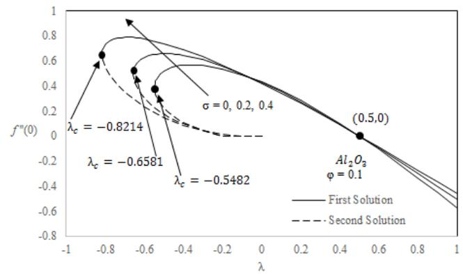
**Fig. 6.** Skin friction coefficient  $f''(0)$  as a function of  $\lambda$  for various values of  $\sigma$ .
