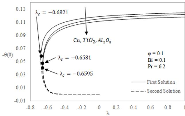
**Fig. 2.** Local Nusselt number coefficient  $-\theta'(0)$  as a function of  $\lambda$  for various various nanoparticles.
