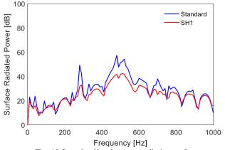
Fig. 18 Sound radiated power, radiating surface
