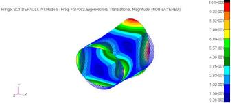
Fig. 12 Structural frame: third mode shape
