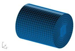
Fig. 9 Fluid cavity domain
