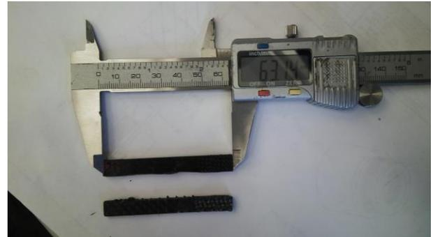
Fig. 3 Composite specimens analyzed
