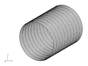
Fig. 5 Fuselage FE Model
