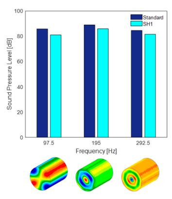
Fig. 13 BPF noise level reduction
