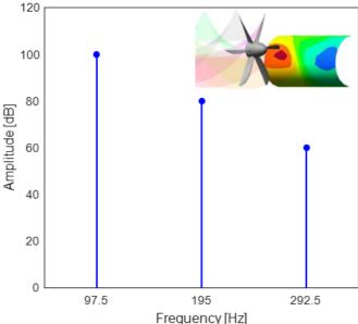
Fig. 7 Propeller tonal load, BPF
