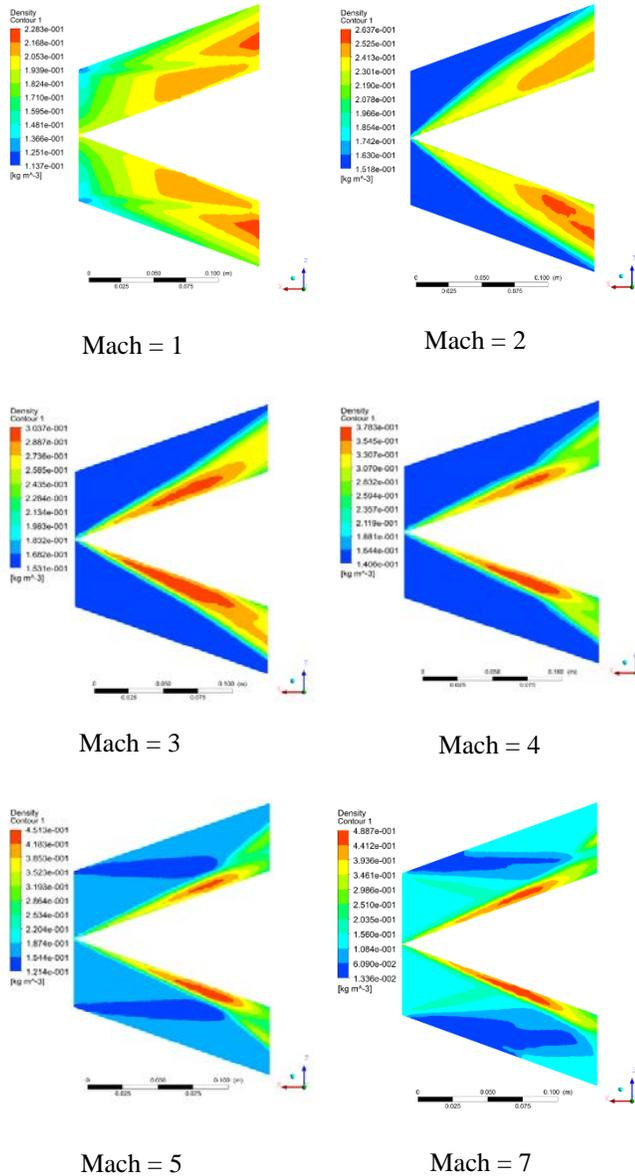
Fig. 2: Contour plot of density for flow over 20° half angle cone at different Mach
