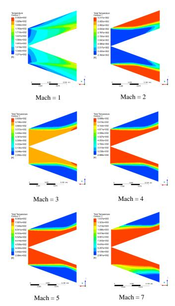
Fig. 5: Contour plot of temperature for flow over 20<sup>0</sup> half angle cone at different Mach
