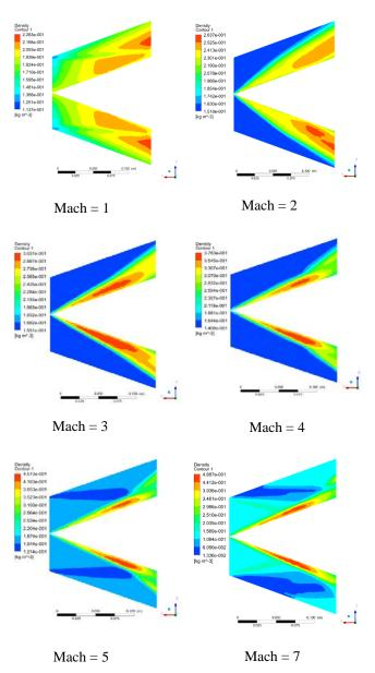
Fig. 2: Contour plot of density for flow over  $20^0$  half angle cone at different Mach
