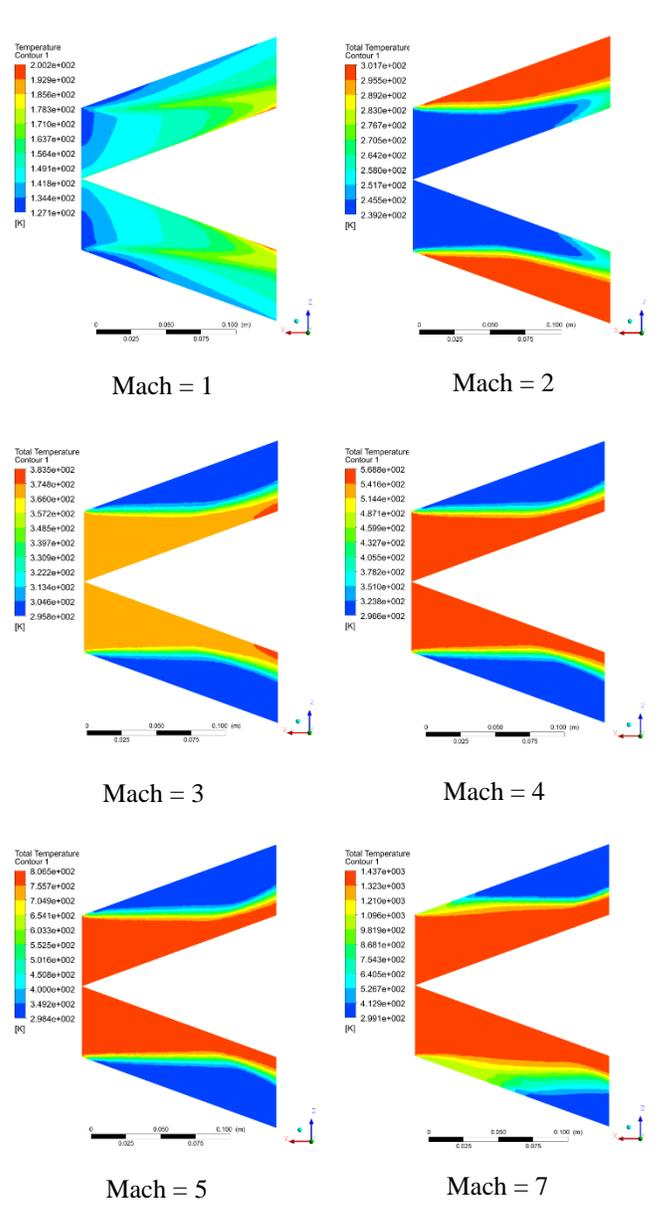
Fig. 5: Contour plot of temperature for flow over 20° half angle cone at different Mach
