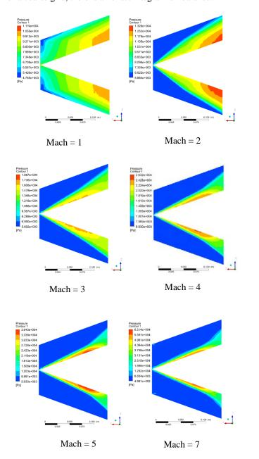
Fig. 4: Contour plot of velocity for flow over  $20^0$  half angle cone at different Mach
