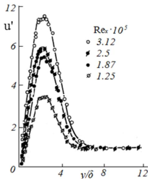
Fig.2 Distribution of the low-frequency longitudinal velocity on the boundary layer for different Reynolds numbers,  $Re_x$  [10]
