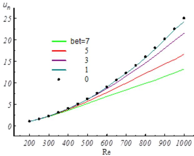
Fig. 11. Dependences of normalized velocity perturbations amplitudes on the Reynolds number at  $M=0.2$  and different values  $bet=\beta \cdot 10^4$
