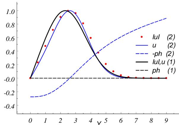
Fig. 7 Distributions of maximum,  $|u|$ , and actual,  $u$ , values of velocity perturbations and a phase shift on a boundary layer at  $Re=200(1)$  and  $10^3(2)$  ( $M=0.2, \beta=7 \cdot 10^{-4}$ )
