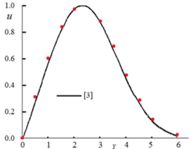
Fig. 3 Comparison of calculation results ( $M=0.2$ ) of the longitudinal velocity distribution with data of [7] ( $M=0$ )
