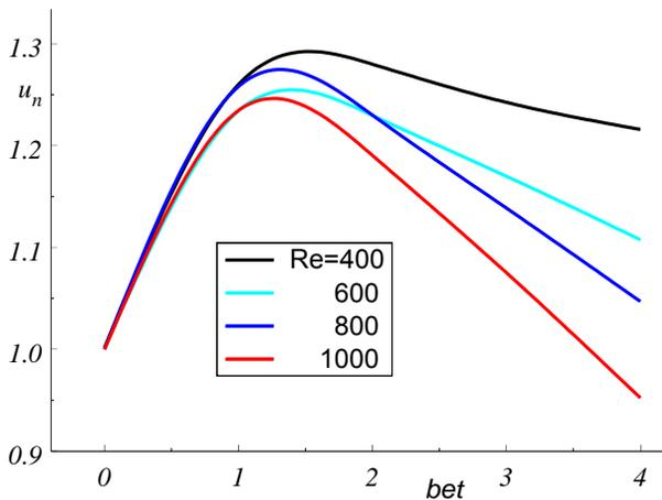
Fig. 12. Dependences of normalized velocity perturbations amplitudes on wave number at  $M=0.2$  and different values  $Re$
