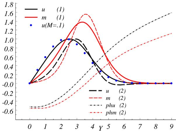
Fig. 8 Distributions  $u, m, ph$  on a boundary layer at  $M=2$ .  $Re=200$  (1),  $10^3$  (2);  $\beta=7 \cdot 10^{-4}$
