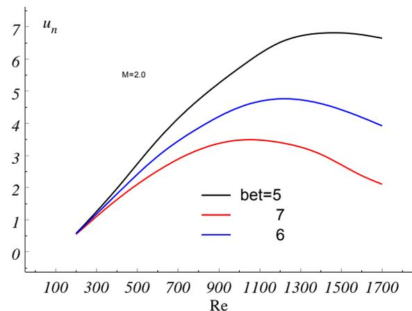
Fig. 14 Dependences of velocity perturbations amplitudes,  $u$ , on the Reynolds number at  $M=2$  and different values  $bet=\beta \cdot 10^4$
