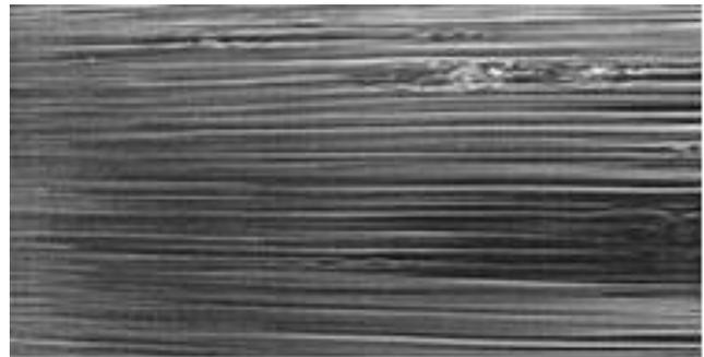
Fig.1 Flow visualization of streaky structures in boundary layers affected by free-stream turbulence [5]
