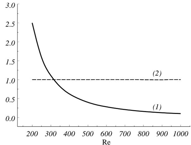
Fig. 4 Dependence of a rate amplification  $\alpha_i$  (1) and (2) on a Reynolds number,  $M=0.2$
