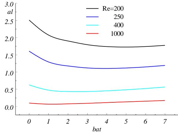
Fig. 10 Decrements dependences on a lateral wave number at  $M=2$  ( $al = \alpha_i \cdot 10^5$ ,  $bat = \beta \cdot 10^4$ ).
