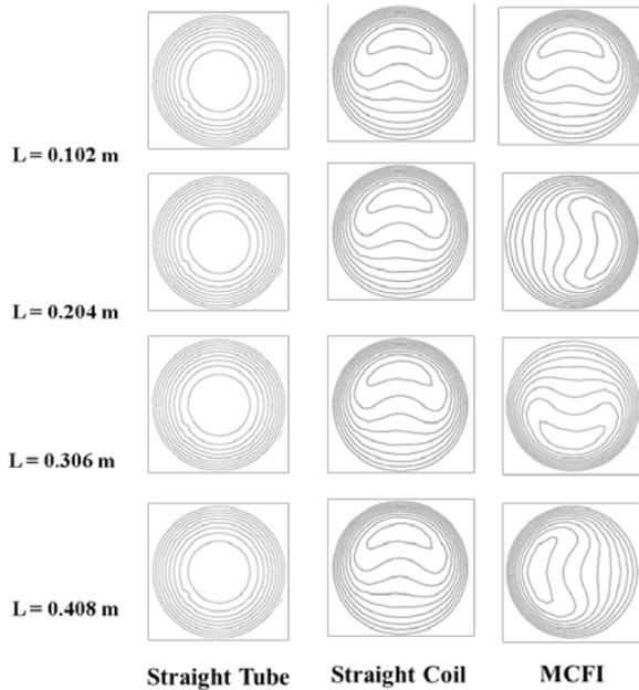
Fig. 4 Velocity profile in MCFI with ID 0.8 mm
