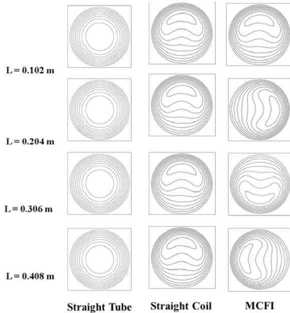
Fig. 4 Velocity profile in MCFI with ID 0.8 mm
