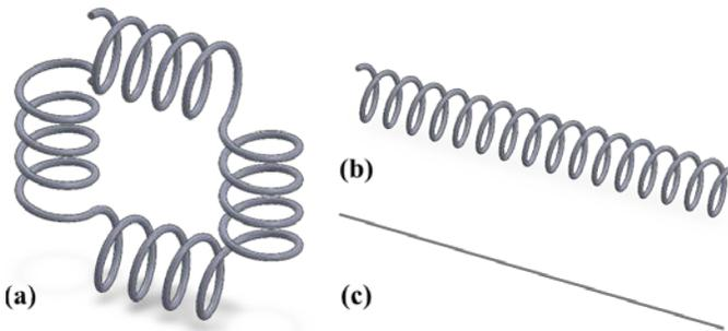
Fig. 1 Geometry design of (a) MCFI, (b) straight coil, and (c) straight tube with equivalent tube diameter and length
