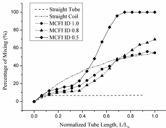
Fig. 6 Mixing plot for MCFI in comparison to straight tube and straight coil
