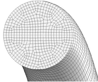
Fig. 2 Mesh topology at the inlet extended throughout the geometry
