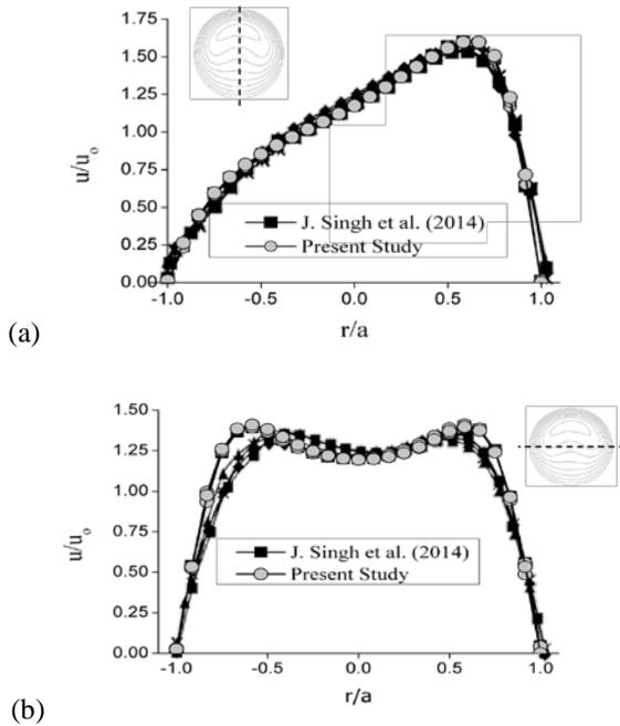
Fig. 3 Comparison of velocity profile in MCFI with data from literature for (a) vertical and (b) horizontal centerline
