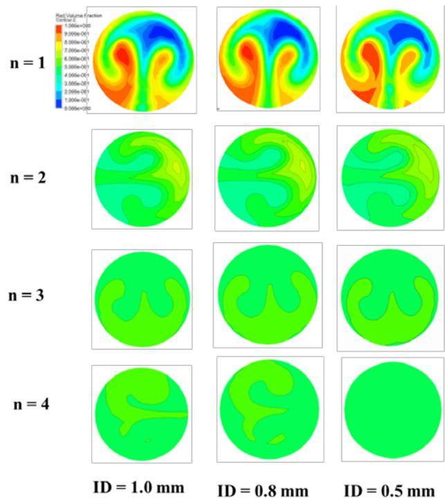
Fig. 5 Cross sectional mass fraction contour for MCFI
