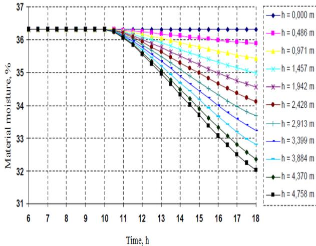
Fig. 3 Behavior of the lateritic mineral moisture distribution in the west slope, from the base to the drying surface.
