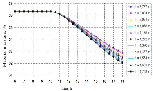
Fig. 5 Behavior of the lateritic mineral moisture distribution in the west slope depending on the drying thickness.
