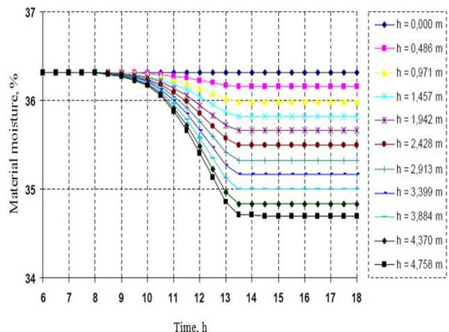
Fig. 2 Behavior of the lateritic mineral moisture distribution in the east slope, from the base to the drying surface.
