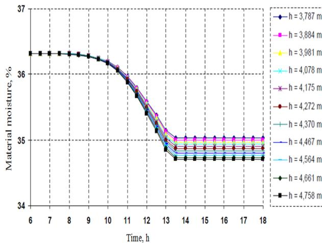
Fig. 4 Behavior of the lateritic mineral moisture distribution in the eastern slope depending on the drying thickness.
