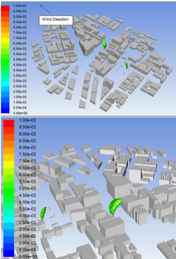
Fig.11 Concentration Profile (Iso surface of 0.005 Dilution Factor)
