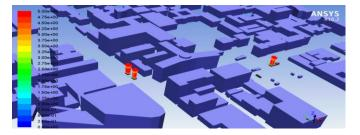
Fig.6 Velocity Vector (m/s) at the smoke Sources
