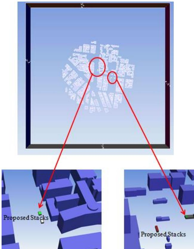
Fig.2 Geometry for CFD Modelling
