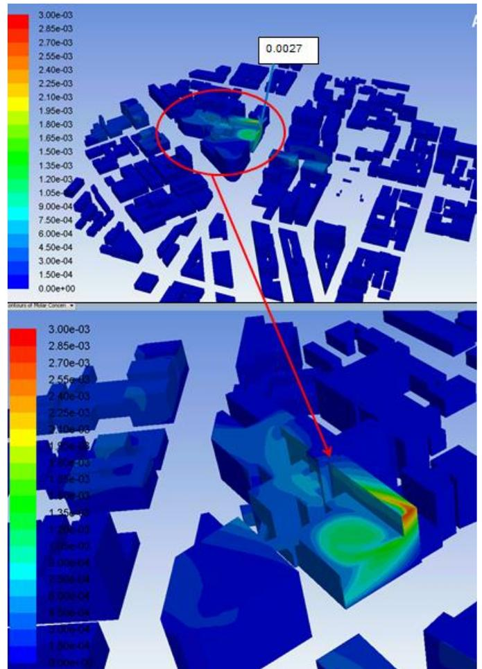
Fig.9 Concentration Profile (Dilution Factor) on the Facades of Buildings
