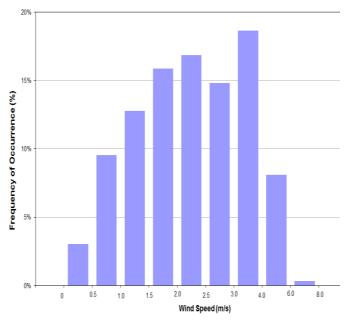
Fig.1 G Wind speed Frequency Distribution for the Project Site, as predicted by CALMET for one Calendar Year
