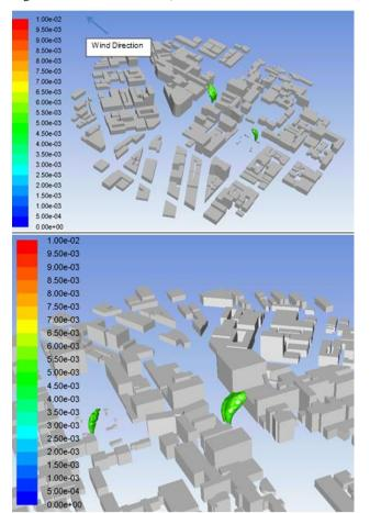
Fig.11 Concentration Profile (Iso surface of 0.005 Dilution Factor)
