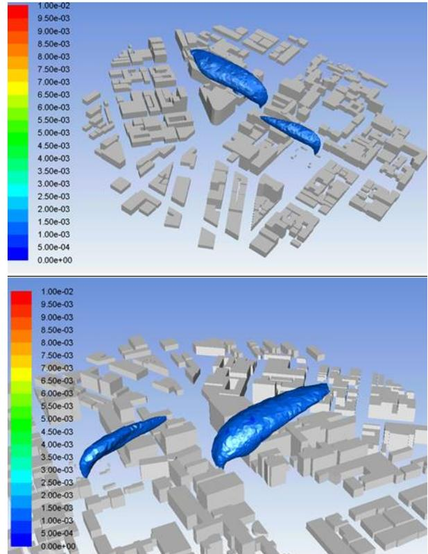
Fig.12 Concentration Profile (Iso Surface of 0.001 Dilution Factor)
