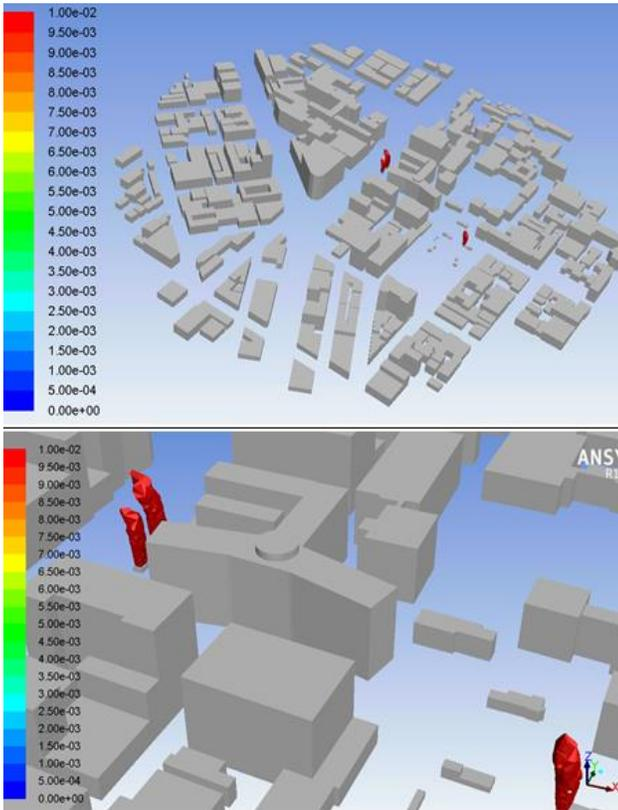
Fig.10 Concentration Profile (Iso Surface of 0.01 Dilution Factor)
