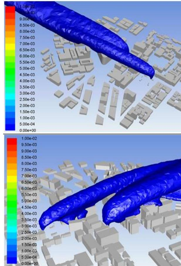
Fig.13 Concentration Profile (Iso Surface of 0.001 Dilution Factor)
