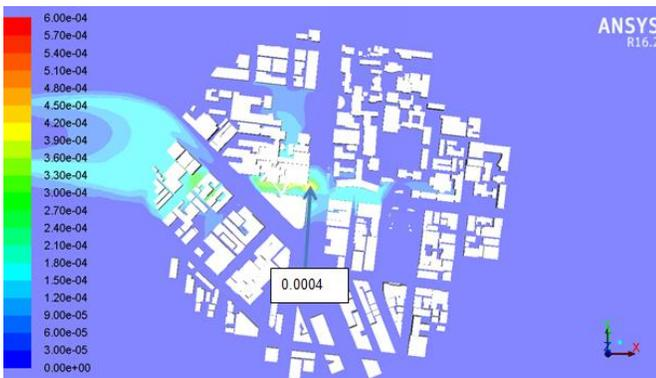
Fig.8 Concentration Profile (Dilution Factor) on the Ground Level
