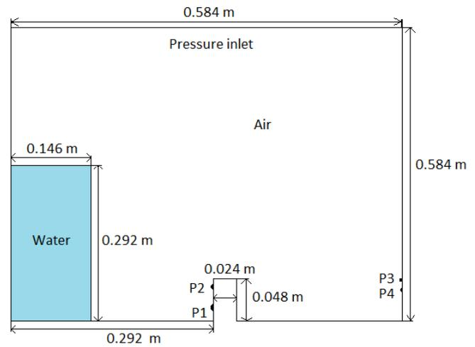
Figure 7 – The geometry of simulation model.
