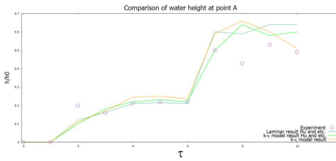
Figure 2 - Comparison of the water height  $h_1$  at point A with numerical simulation results and experimental data [22].
