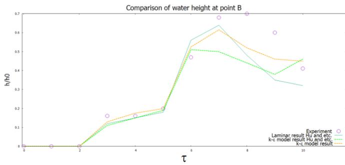
Figure 3 - Comparison of the water height  $h_2$  at point B with numerical simulation results and experimental data [22].
