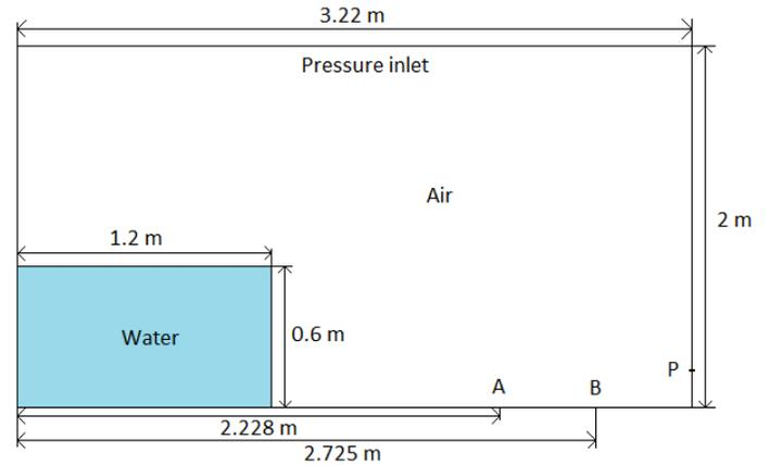
Figure 1 – The geometry of simulation model.
