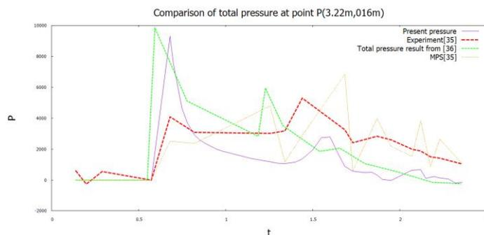
Figure 5 – Comparison of pressure impact against downstream wall at point  $P(3.22m,0.16m)$  with numerical simulation results and experimental data.
