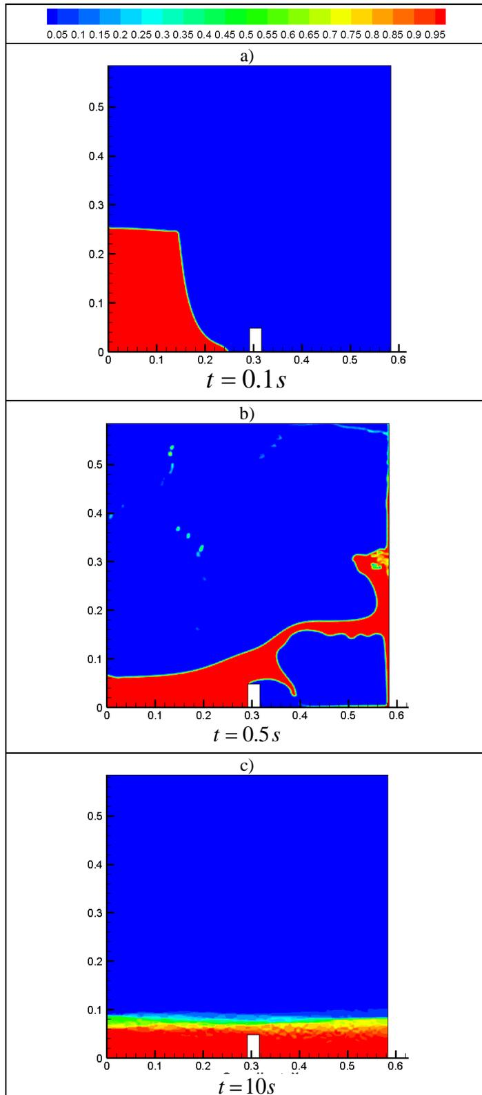
Figure 10 – Impact of a water flow on a rectangular obstacle.
