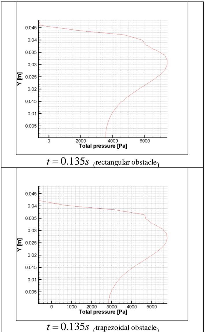
Figure 13 - Impact of a water flow on a rectangular and trapezoidal obstacle, pressure fronts.
