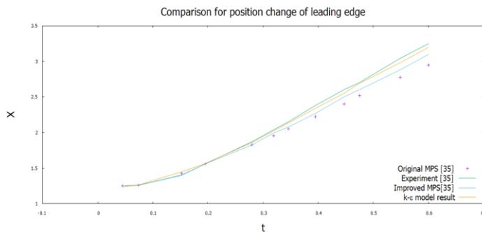
Figure 4 - Comparison of the water front with numerical simulation results and experimental data [23].
