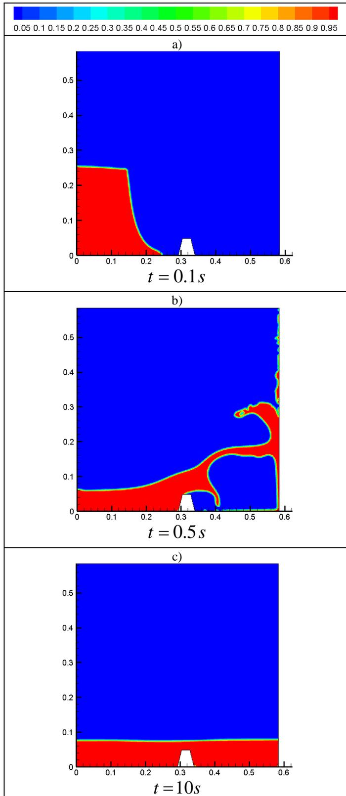
Figure 12 - Impact of a water flow on a trapezoidal obstacle.
