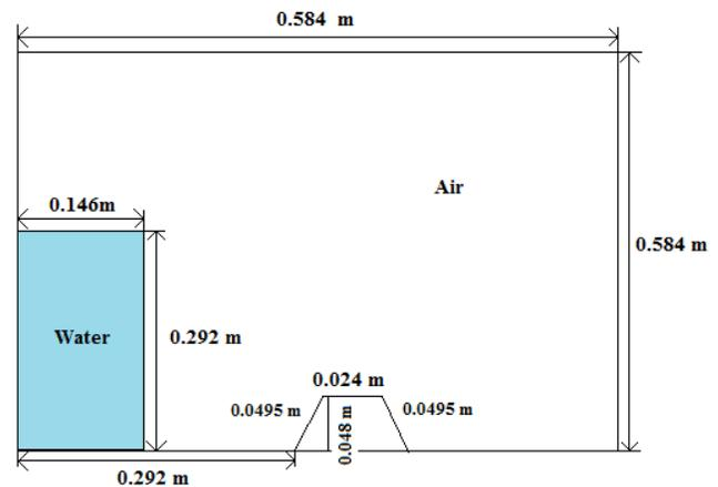
Figure 11 – The geometry of the simulation model.
