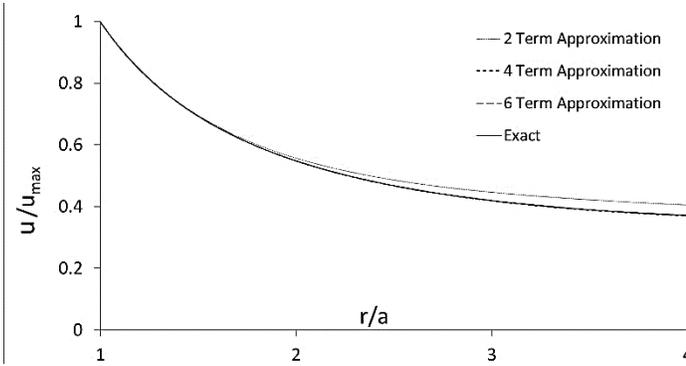
Fig. 5 comparison of radial displacements for inner pressure case
