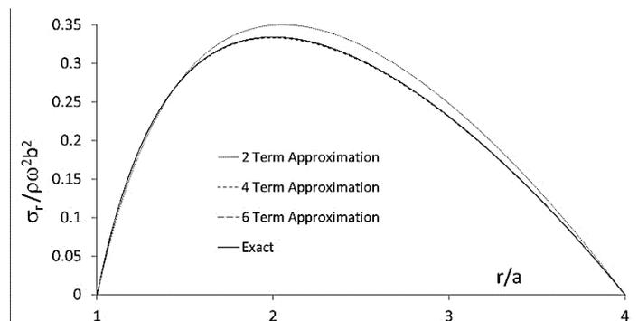
Fig. 9 comparison of radial stresses for rotating disk case
