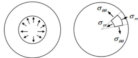
Fig. 1 cylinder under internal pressure and stress components
