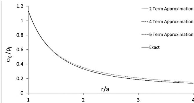
Fig. 4 comparison of tangential stresses for inner pressure case
