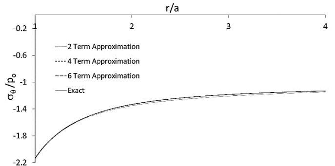
Fig. 7 comparison of tangential stresses for external pressure case
