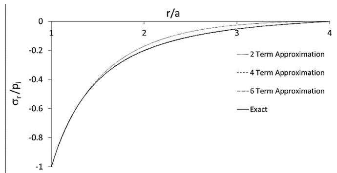
Fig. 3 comparison of radial stresses for inner pressure case
