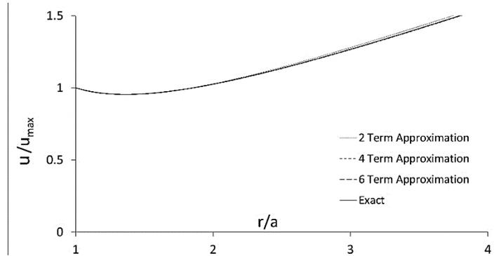
Fig. 8 comparison of radial displacements for external pressure case
