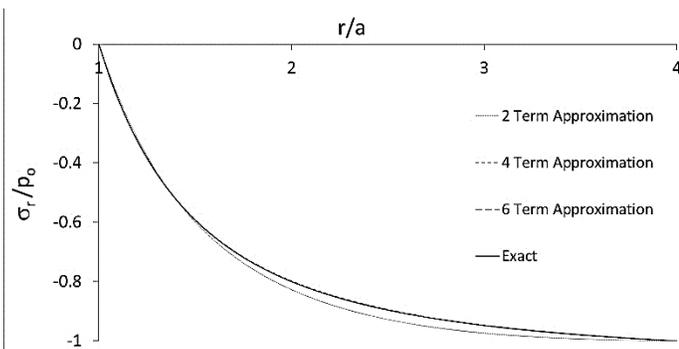
Fig. 6 comparison of radial stresses for external pressure case
