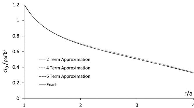
Fig. 10 comparison of tangential stresses for rotating disk case
