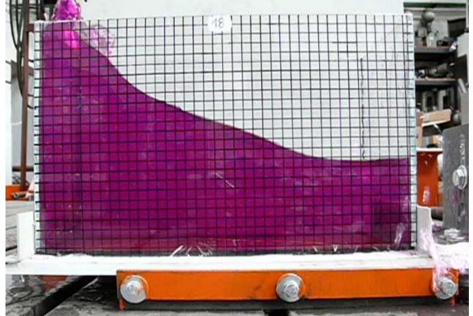
Fig. 15 the fluid splash out from rectangular tank for 15 cm water filling
