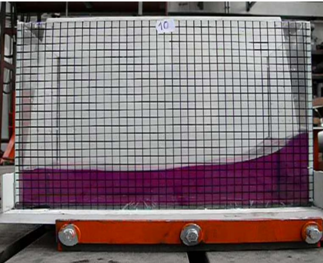
Fig. 12 the fluid wave in rectangular tank for 5 cm water filling
