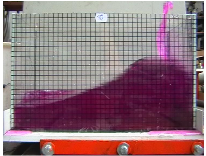
Fig. 11 the fluid flow in rectangular tank for 5 cm water filling
