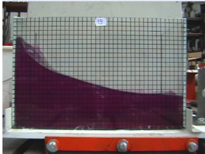
Fig. 14 the fluid wave in rectangular tank for 10 cm water filling
