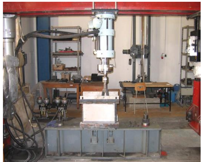
Fig. 14 illustration of the loading test of the steel mechanical anchors with the cyclic tension force
