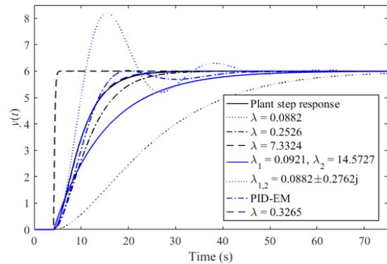
Fig. 7 Step response of (27) vs. control responses
