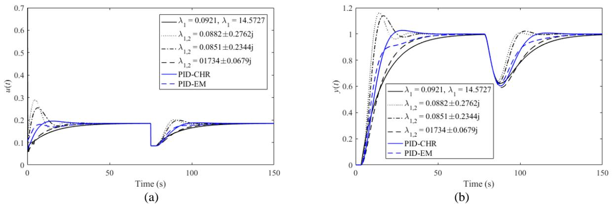
Fig. 13 Selected perturbed control responses  $u(t)$  (a),  $y(t)$  (b) according to (39) – Example 2,  $m_2(s)$
