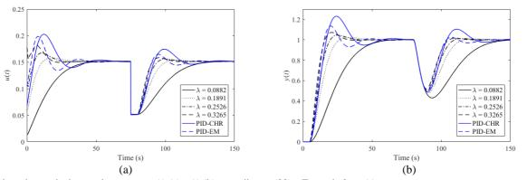
Fig. 10 Selected perturbed control responses u(t) (a), y(t) (b) according to (38) – Example 2,  $m_1(s)$
