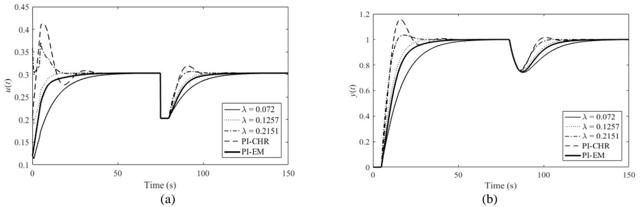
Fig. 5 Selected perturbed control responses  $u(t)$  (a),  $y(t)$  (b) according to (38) – Example 1
