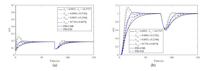
Fig. 13 Selected perturbed control responses u(t) (a), y(t) (b) according to (39) – Example 2,  $m_2(s)$
