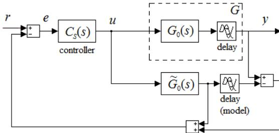
Fig. 1 Smith predictor (delay compensator) scheme
