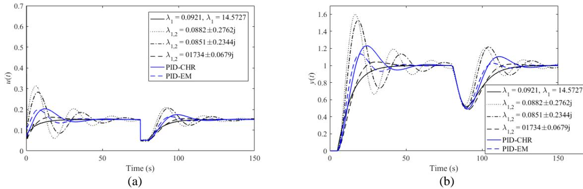
Fig. 11 Selected perturbed control responses  $u(t)$  (a),  $y(t)$  (b) according to (38) – Example 2,  $m_2(s)$
