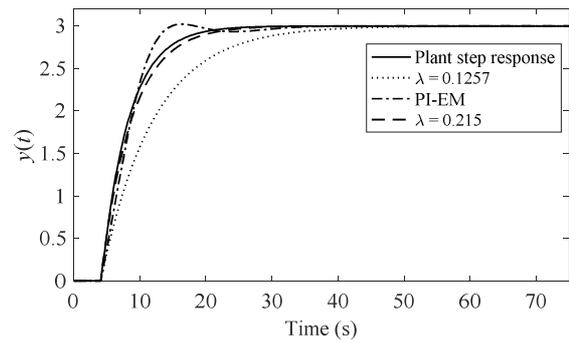
Fig. 3 Step response of (16) vs. control responses
