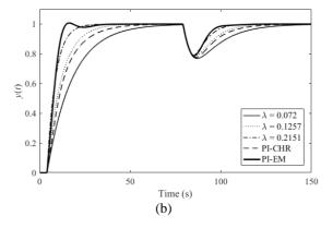
measures for the calculated controllers are benchmarked against each other in Table II, and control responses are displayed in Fig. 5. For perturbation (38), a very good choice is represented by the found balanced value  $\lambda = 0.2151$  (in the sense of EM). A lower value of  $\lambda$  gives a slower control response, while the direct PI design via the CHR method yields an aggressive yet not very fast response.
