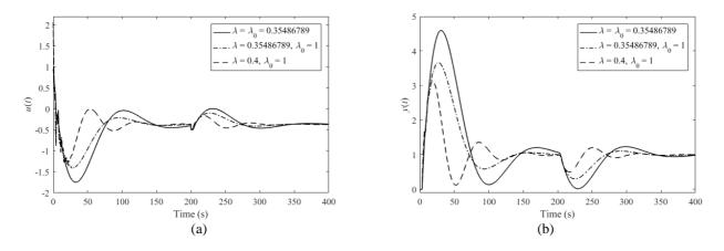
Fig. 16 Selected perturbed control responses u(t) (a), y(t) (b) according to (39) – Example 3
