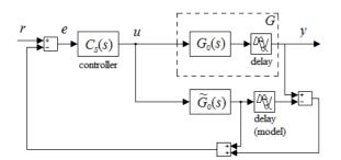
Fig. 1 Smith predictor (delay compensator) scheme
