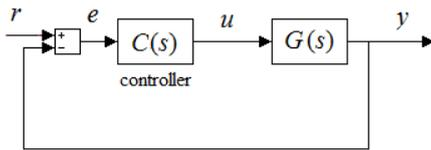
Fig. 2 Simple negative feedback loop scheme
