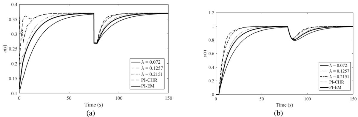
Fig. 6 Selected perturbed control responses  $u(t)$  (a),  $y(t)$  (b) according to (39) – Example 1
