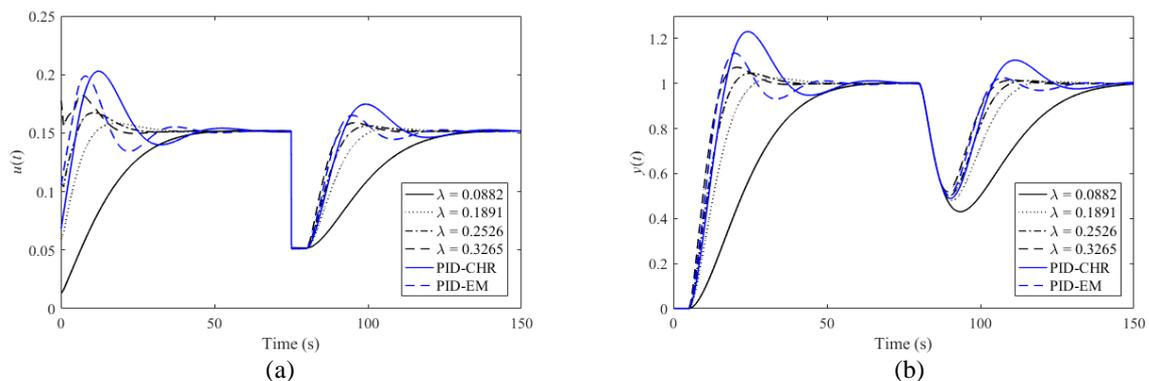
Fig. 10 Selected perturbed control responses  $u(t)$  (a),  $y(t)$  (b) according to (38) – Example 2,  $m_1(s)$
