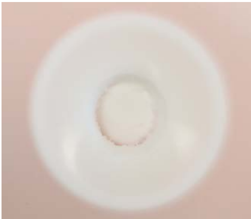
Fig. 10 PP deformation after-drop weight impact test at 230 J
