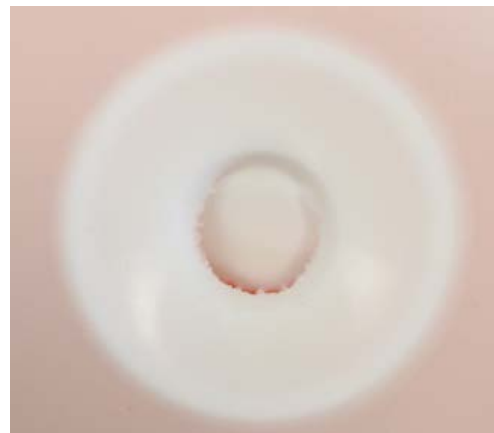
Fig. 8 PP deformation after drop-weight impact test at 100 J
