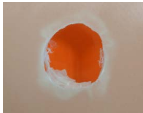
Fig. 7 PP30GF deformation after drop-weight impact test at 100 J
