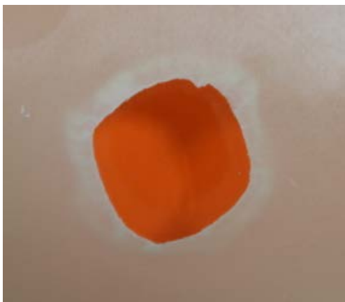
Fig. 5 PP30GF deformation after drop-weight impact test at 30 J
