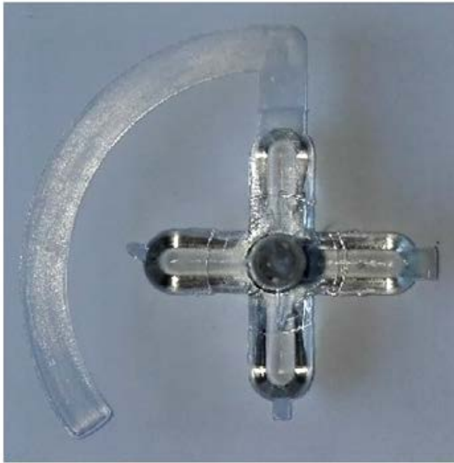
Fig. 9. Real testing sample (material PC, injection pressure 500 bar).
