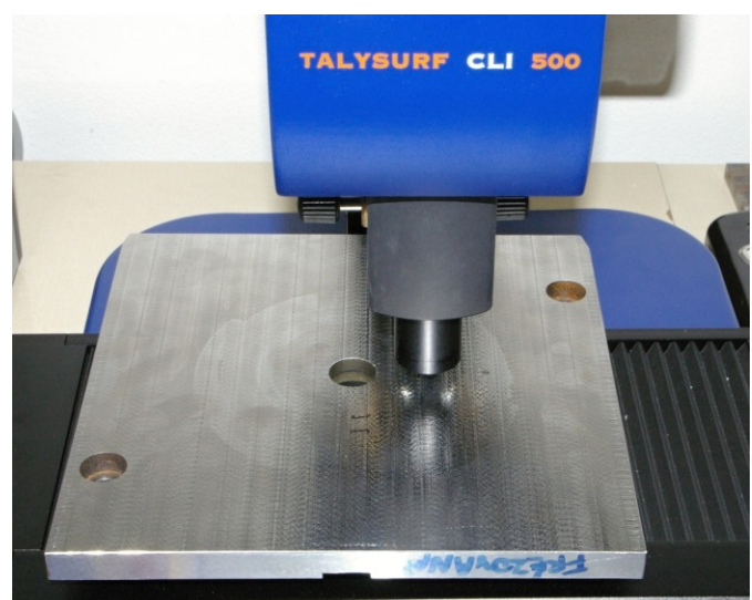
Fig. 5. Testing plate surface scanning by Talysurf CLI 500.
