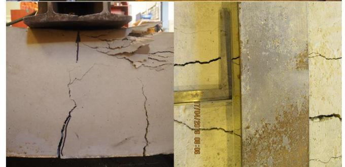
Fig. 12 the composite beam under the load of 400 kN; visible destruction at the point, where the force was applied; destruction in the middle of the beams span seen from the bottom of the beam
