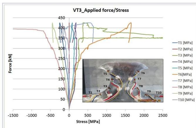
Fig. 13 the force/stress diagrams, test specimen VT1, VT2, VT3
