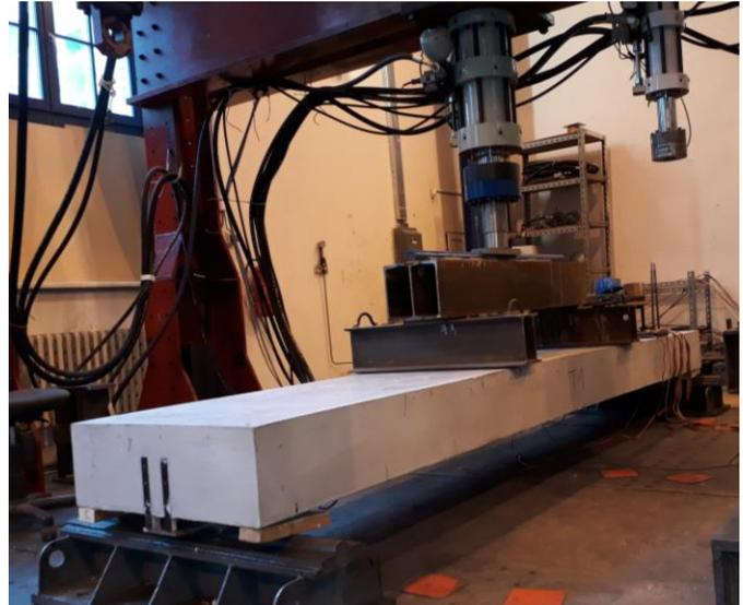
Fig. 11 four-point bending test, simply supported beam with visible shrinkage cracks
