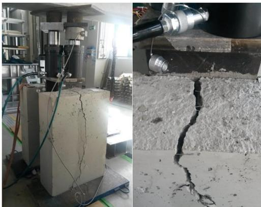
Fig. 4 push-out test, the failure of the specimen
