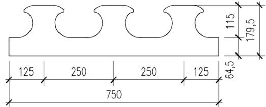
Fig. 5 dimensions of the steel strip
