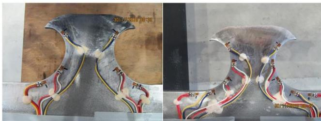
Fig. 7 the location of strain gauges
