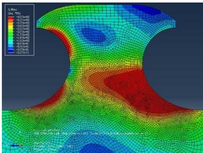
Fig. 6 stress distribution under the load of 100 kN
