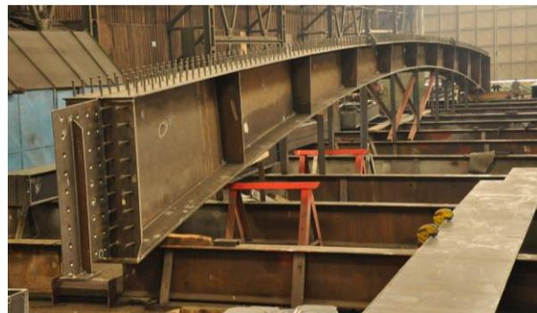
Fig. 1 Pcb girder for pedestrian bridge in Czech Republic
