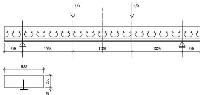
Fig. 10 the layout of the four-point bending test, beam's cross section
