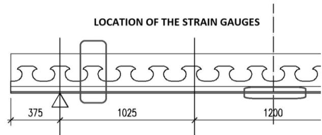
Fig. 8 the position of strain gauges
