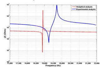
Figure 4. Impedance curve from analytical and experimental
