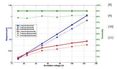
Figure 5. Numerical and experimental peak responses and torsionality for different excitation voltages.
