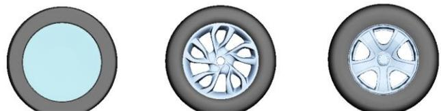
Fig. 3. Rim designs for CFD simulations
