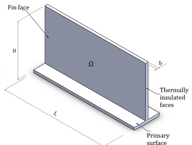
Fig. 1: Boundary and domain of fins.
