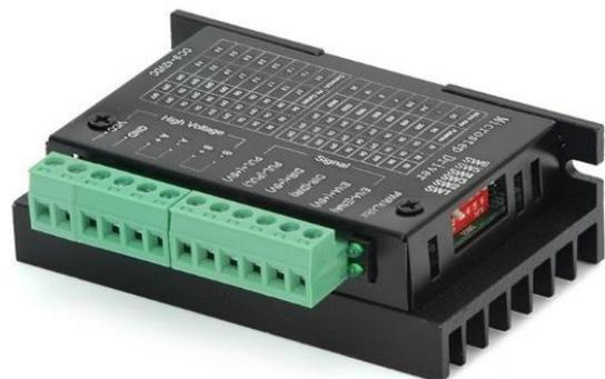
Fig. 5. TB6600 stepper motor driver
