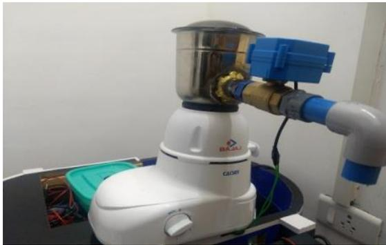
Fig. 1. Mixer-Grinder with Motorized Valve
