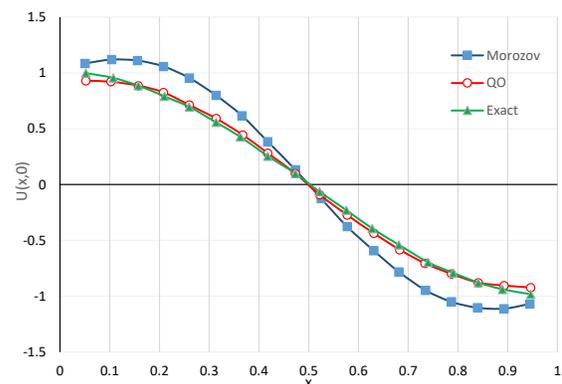
Fig. 4 Comparison of the approximate solution obtained using Quasi-Optimality and Morozov's regularization parameter with the exact solution for noise = 3% and  $\tau = 0.1$  and  $n = 54$  and  $f = 54$
