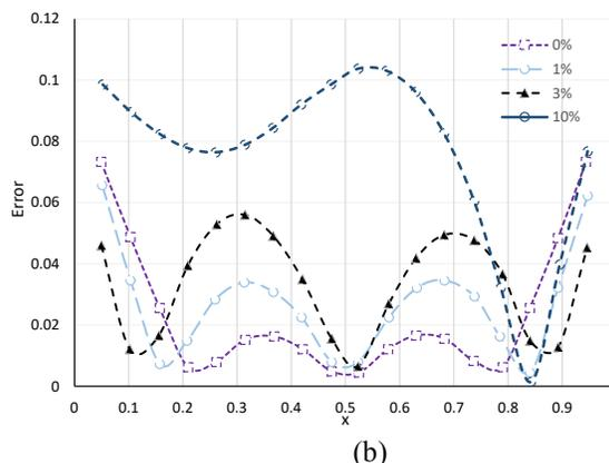
Fig. 5 The error in the collocation points on the boundary  $t = 0$  for  $n = 54, f = 54,$  and at different noise levels, a) using the Quasi -optimality criterion b) using the Morozov's discrepancy principle.
