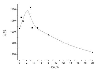
Fig. 4 dependence of elongation at break of Cu/LLDPE samples on nanofiller content
