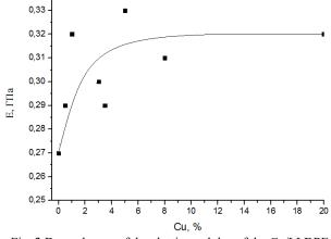
Fig. 2 Dependences of the elastic modulus of the Cu/LLDPE nanocomposite on the filler content
