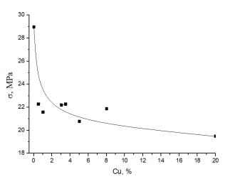
Fig. 3 Dependences of the tensile strength of the Cu/LLDPE nanocomposite on the filler content
