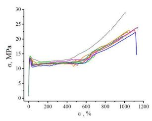
Fig. 1 Stress-Strain curves for initial LLDPE and Cu/LLDPE nanocomposites with different filler contents
