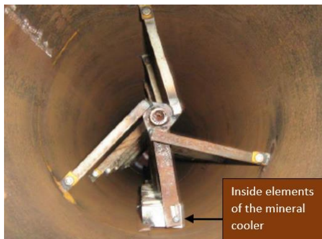
Figure 2. Inside element of the mineral cooler
