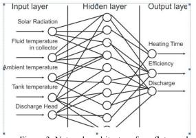
Figure 3. Network architecture for a flat panel solar collector with a heat pump
