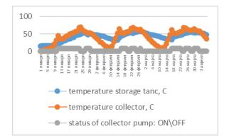
Figure 9. Ambient and manifold and reservoir temperatures with pump operating mode
