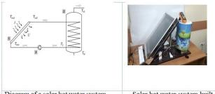
Diagram of a solar hot water systemSolar hot water system builtFigure 1. Solar hot water system. 1 - flat solar collector; 2 -<br/>storage tank with a heat exchanger; 3 - pump
