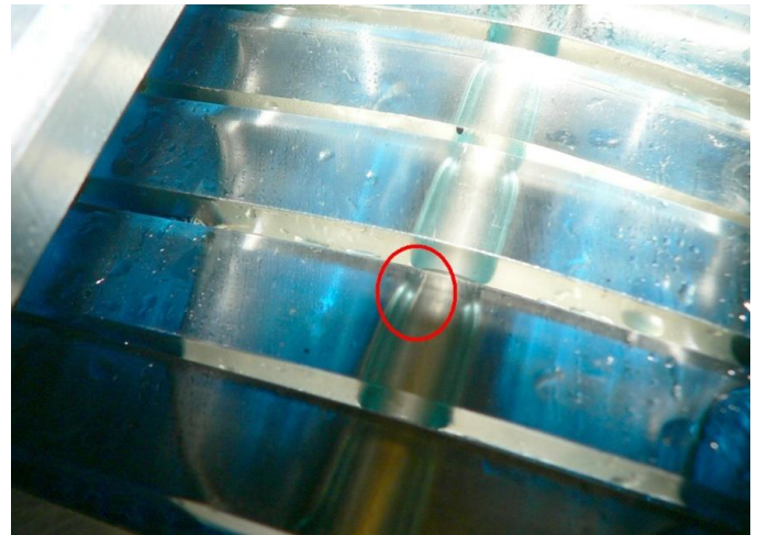
Fig. 17 Irradiated PA11 specimens placed in the ethyleneglykol environment after 72 hours
