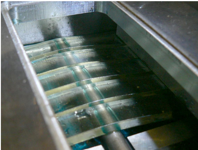
Fig. 14 Non-irradiated PA11 specimens placed in the ethyleneglykol environment after 24 hours
