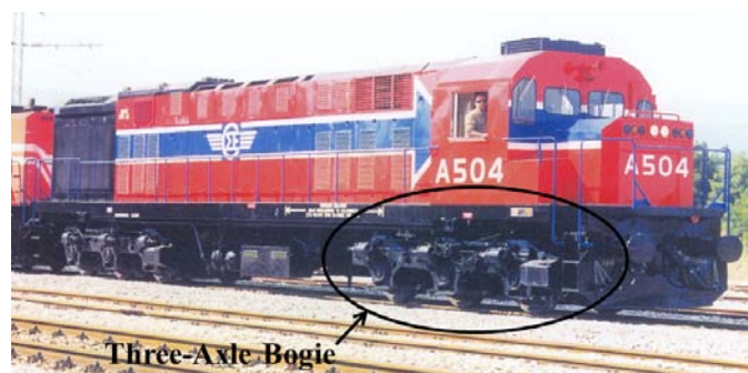
Figure 1 Diesel Locomotive of the Greek railways with three-axle bogies, on a railway track. The three-axle bogie is marked with the black ellipse.
