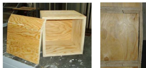
Fig. 4 block specimens after the failure
