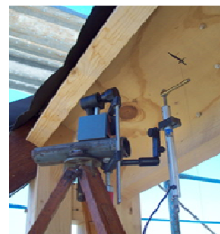
Fig. 9 displacement transducers utilized in the tests on the real structure; (a) touch transducer at the key section; (b) inductive transducer at a shoulder.
