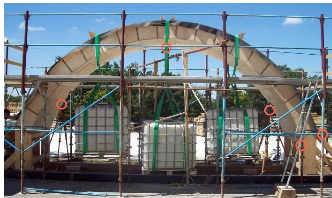
Fig. 7 tested arch: details with the low tanks of the positioning of the displacement transducers
