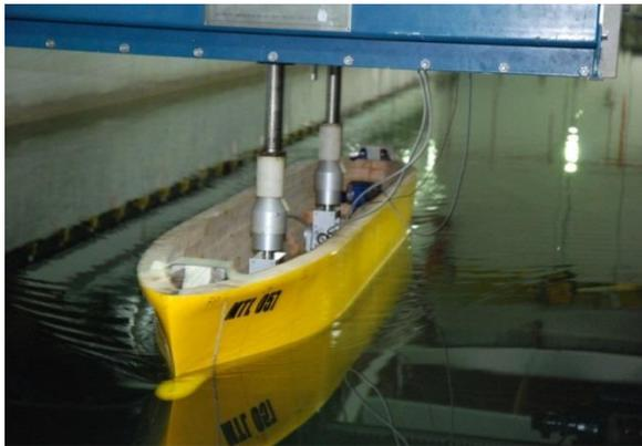
Fig. 7 Ship model test in open water
