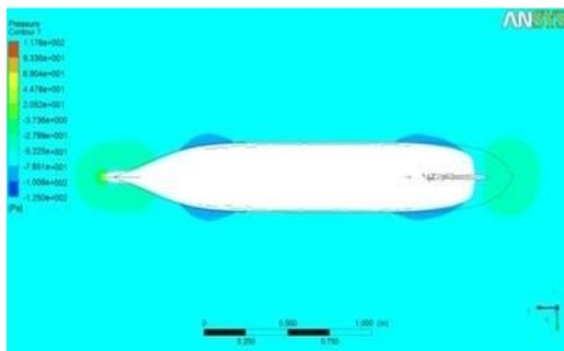
Fig. 19 Pressure contours around the ship in deep water
