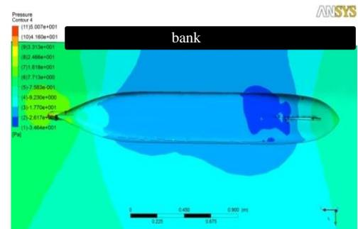
Fig. 20 Pressure contours around the ship in confined water
