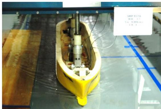
Fig. 8 Ship model in testing situation to study the effect of bank and shallow water
