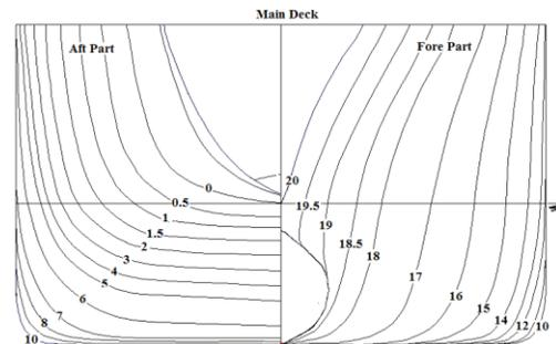
Fig. 1 Body plan of the LNG ship
