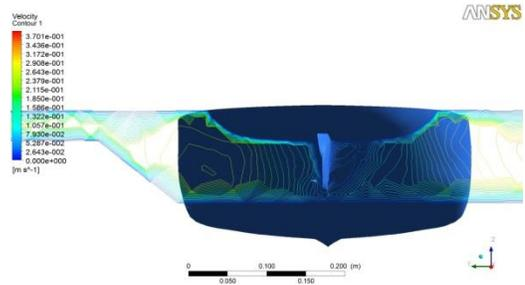
Fig. 14 Velocity line contours at inflow propeller plane
