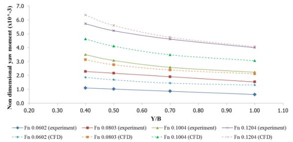
Fig. 9 Effect of ship speed on yaw moment at H/D =1.6
