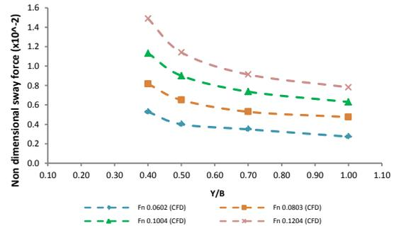
Fig. 10 Effect of ship speed on sway force at H/D =1.6
