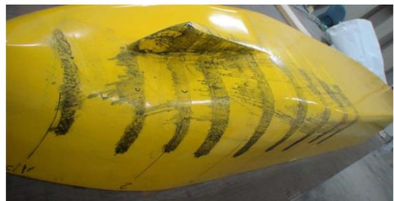
Fig. 11 Paint Smear Test velocity streamlines
