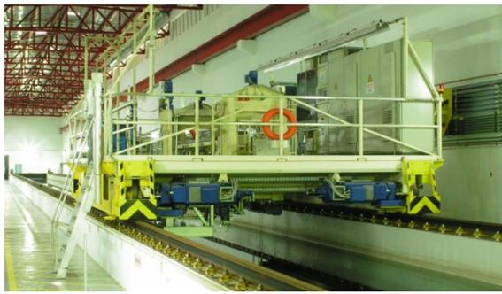
Fig. 6 Towing tank and towing carriage in UTM
