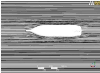
Fig. 17 streamlines around the ship in deep water
