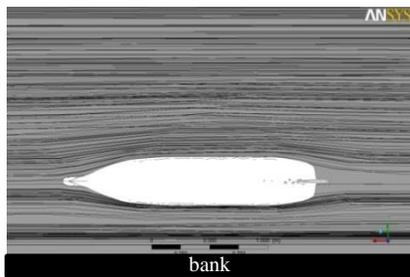
Fig. 18 Streamlines around the ship in confined water
