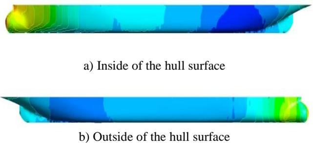
Fig. 16 Measured distributions of pressure coefficients on the hull surface
