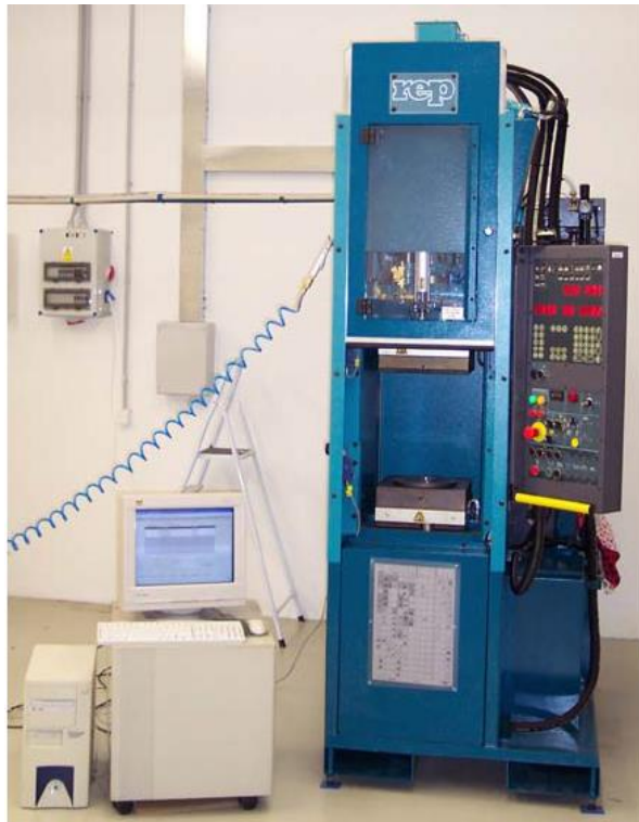
Fig.10 Injection molding machine REP V27/Y125
