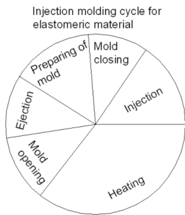
Fig.2 Elastomeric injection molding cycle
