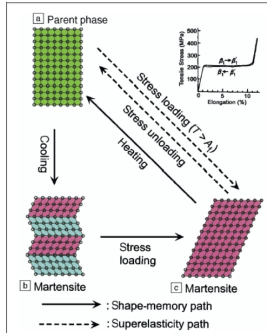
Fig.2: Schematic illustration of the mechanism of the shape-memory effect and superelasticity.
