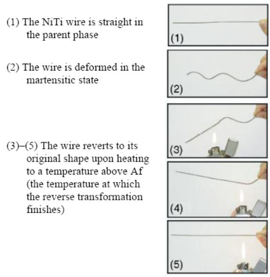
Fig.3: A series of photographs showing the one way shape memory effect for a nickel-titanium wire.
