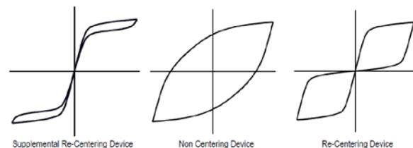
Fig.7. Categories of the types of devices based on SMA.
