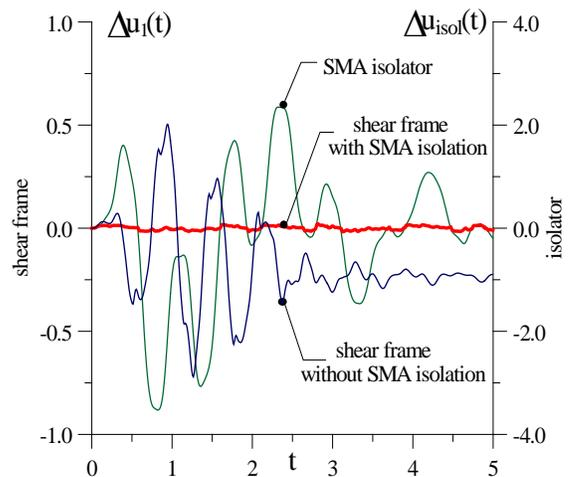
Fig.9: Drift in the shear frame with and without SMA isolation for the 1<sup>st</sup> floor.
