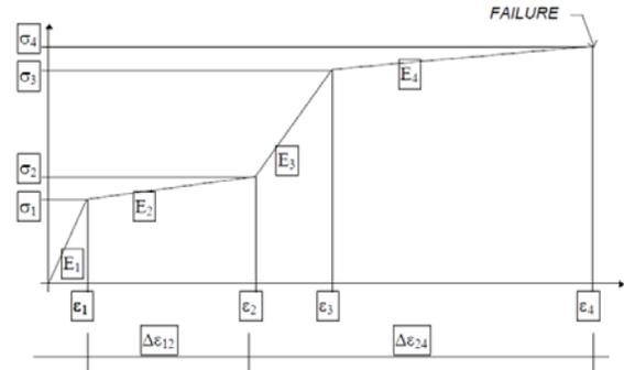
Fig.6: Characteristic quantities defining the mechanical behaviour of SMA.
