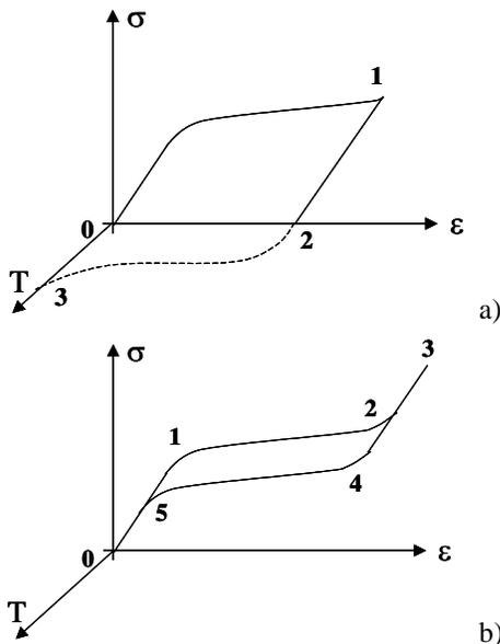
Fig.5: a) Shape memory effect; b) super-elasticity.
