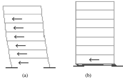
Fig.8: Sketches of the shear frame during the motion: a) structure without SMA isolation, b) structure with SMA isolation.
