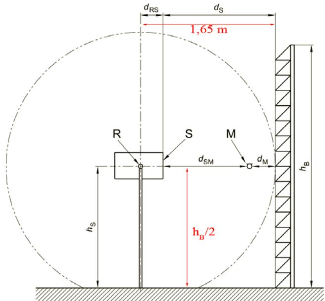
Figure 1. – Sound Reflection geometrical layout according to CEN/TS 1793/5
