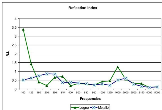
Figure 11 - Reflection Index RI for the two barriers - comparison
