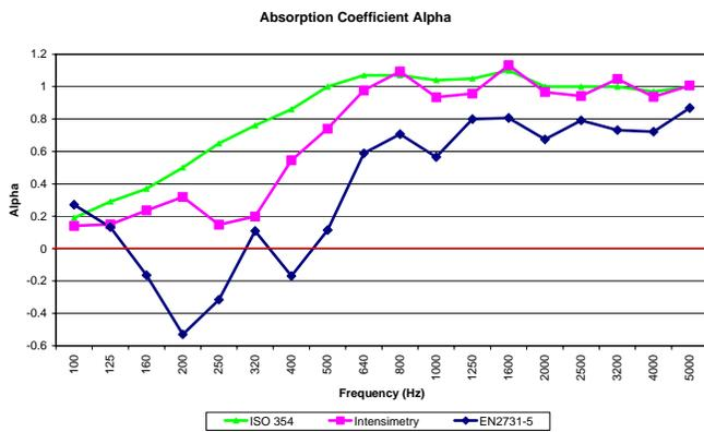
Figure 13. Sound Intensity measurement results (barrier “C”) vs. ISO 354 and CEN/TS 1793/5
