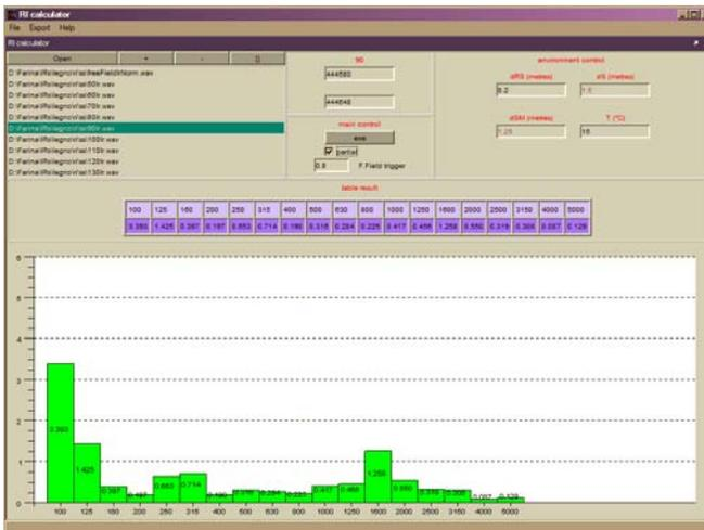
Figure 10 - Wooden barrier - Reflection Index -  $DL_{RI} = 3.41 \text{ [dB]}$
