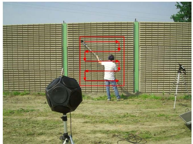
Figure 12. Sound Intensity measurement (manual sweep) of barrier “C”
