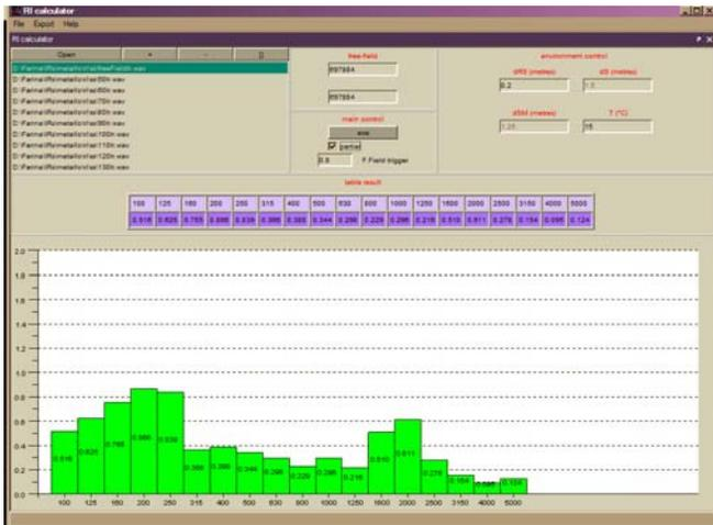
Figure 9 - Steel and PMMA barrier - Reflection Index -  $DL_{RI} = 4.52 \text{ [dB]}$
