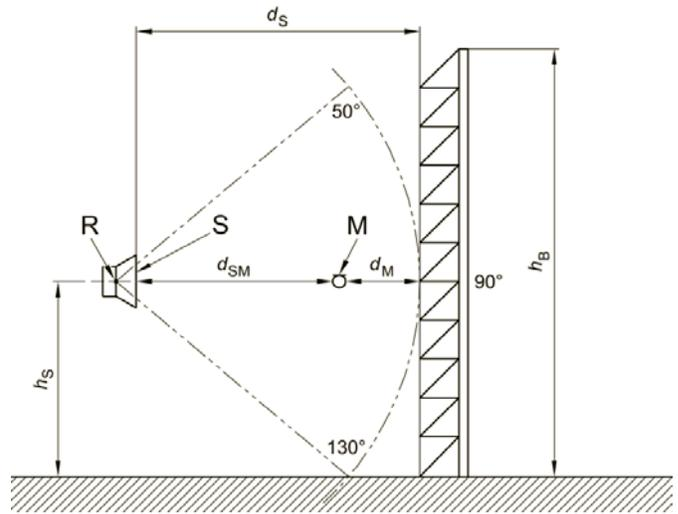
Figure 1. Vertical rotation of the measurement equipment according to CEN/TS 1793/5
