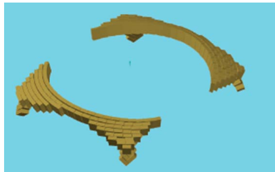
Fig. 15 - Scheme of the collapsed vault, and its standing parts.
