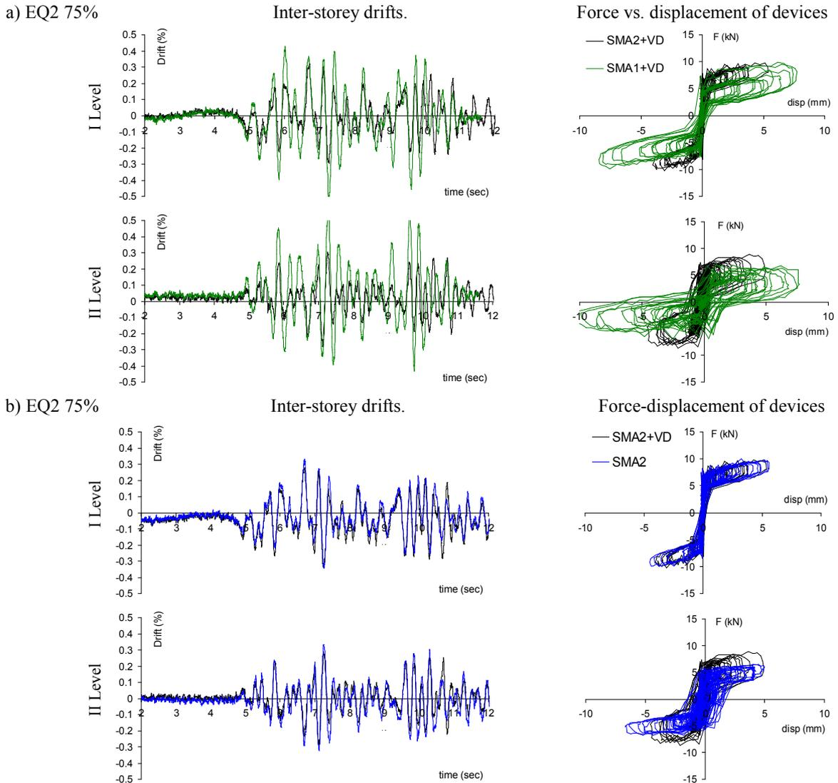
Fig. 8. Comparison of experimental time-histories of drift and force-displacement for visco-recentring devices at the two levels, earthquake n.2, PGA = 75%, between SMA2+VD EBD configurations: a) SMA1+VD; b) SMA2.
