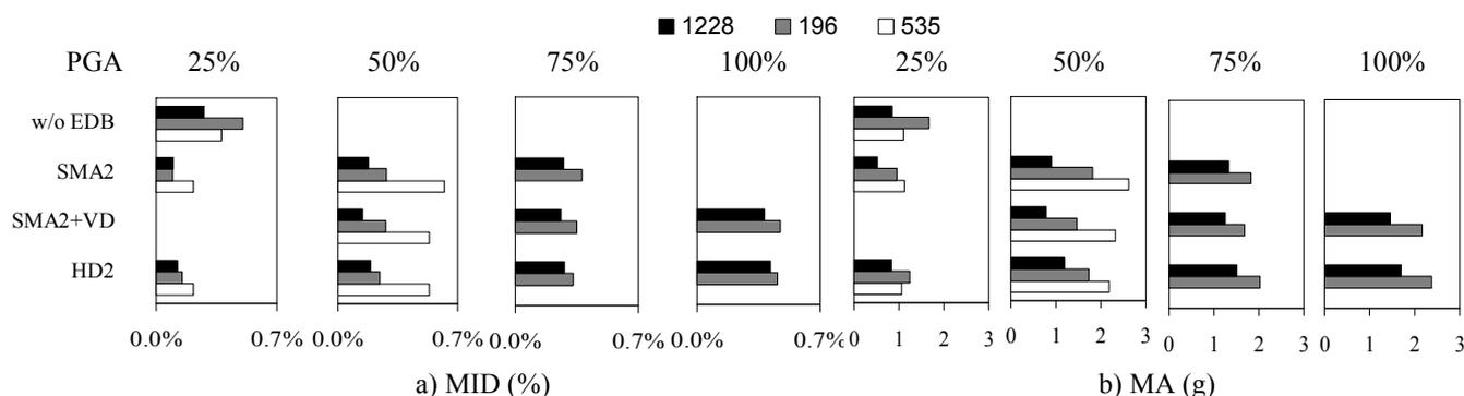
Fig. 11. Experimental results of the frame w/o EDBs and with SMA2, SMA2+VD and HD2 EDBs, earthquakes n. 1, 2 and 3, at PGA = 25%, 50%, 75% and 100%, in terms of: a) MID; b) MA.
