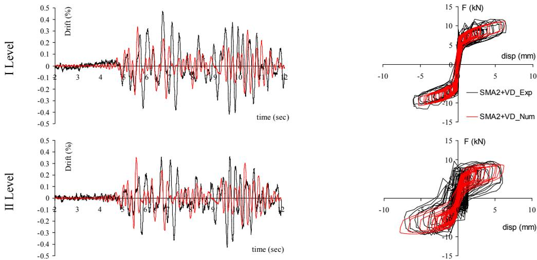
Fig. 9. Experimental and numerical Time-histories of drift and force-displacement of SMA2+VD devices, for earthquake n. 2, PGA =100% PGA 100%.
