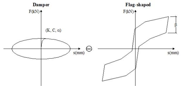
Fig. 6. Sum of models of a) Multilinear elastic (be), b) elasto-perfectly plastic (epp), c) viscous (v), d) flag-shaped model.
