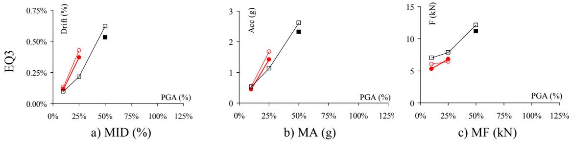
Fig. 7. Experimental results for the frame with SMA1, SMA2, SMA1+VD and SMA2+VD EDBs, for earthquakes n. 1, 2 and 3 at different intensities, in terms of: (a) MID, (b) MA and (c) MF
