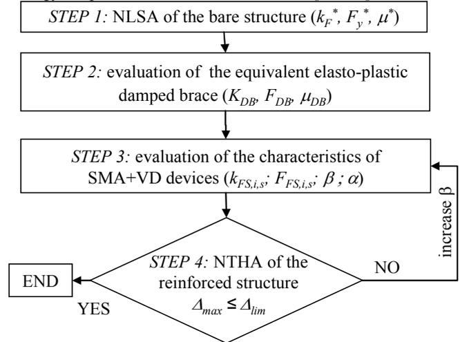
Fig. 2. Flowchart of the design procedure
