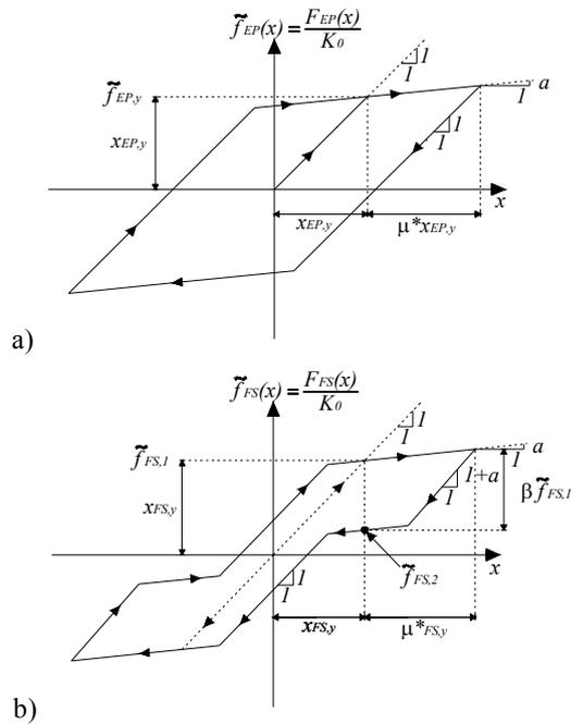
Fig. 1. Equivalent models of (a) Elasto-Plastic (EP) and (b) Flag-Shaped (FS)
