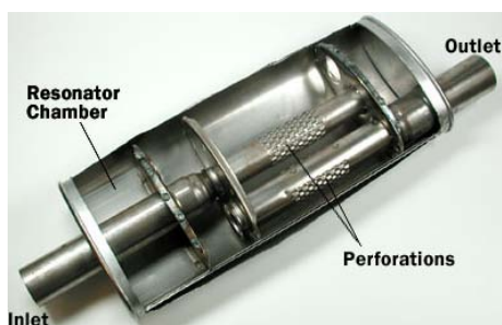
Fig. 1 Typical muffler design [13]
